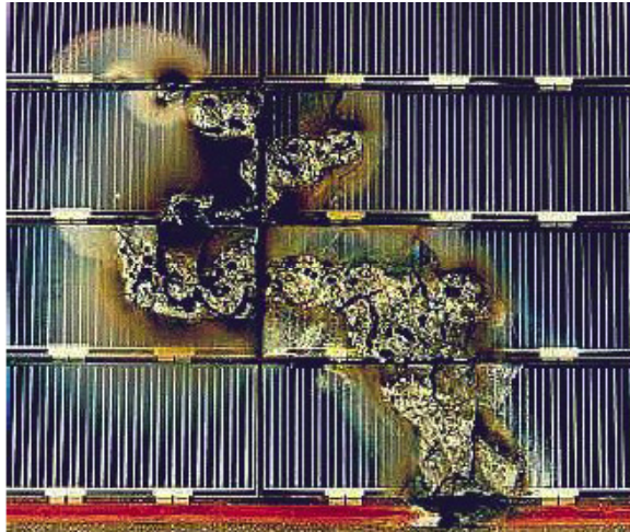
(a) Failure caused by in-flight ESD arcing
