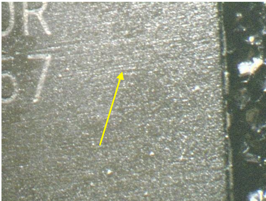
Figure B.6. This image shows a plastic surface after wiping with an acetone swab. Note the horizontal sanding marks in the plastic (yellow arrow).
