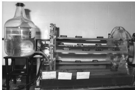
(b) Alternate Immersion Tester
