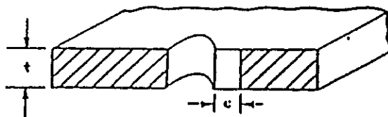
THROUGH CRACK
