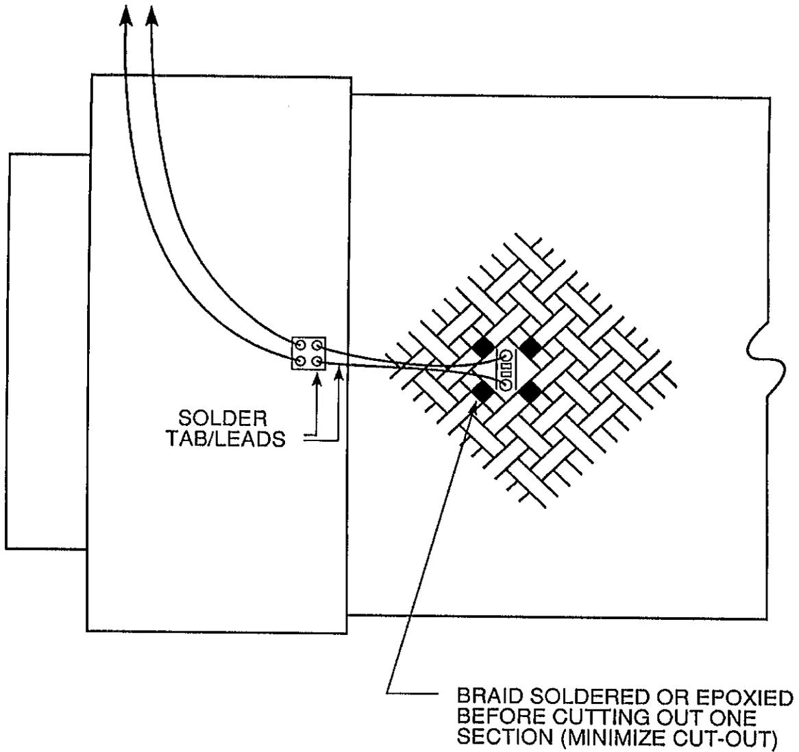
**FIGURE 2. STRAIN GAGE INSTALLATION ON A FLEX HOSE**
