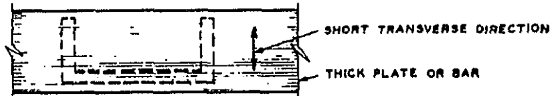
LOCATION OF MACHINED CHANNEL IN PLATE OR BAR
