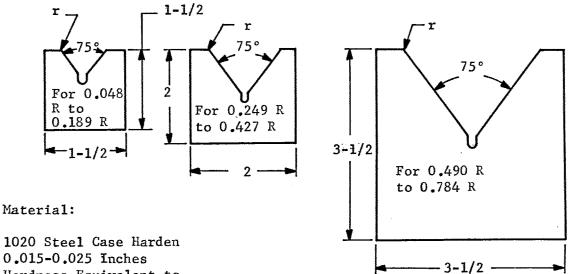
0.015-0.025 Inches Hardness Equivalent to Rockwell C-55 Minimum
