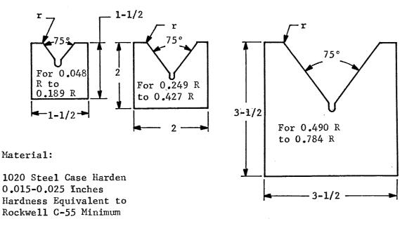
r - .010" Min Radius to Prevent Galling and Binding
