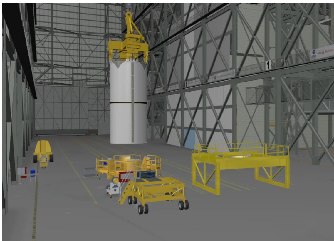
FIGURE 6. SRB Stacking Simulation in the VAB using Light-weight Viewables. Note the VAB Infrastructure
