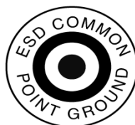
Figure 5-3: ESD Common Point Ground Symbol
