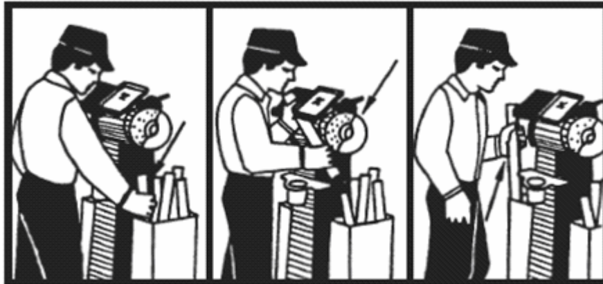
Figure 2. Existing or potential hazards for grinding iron castings.
