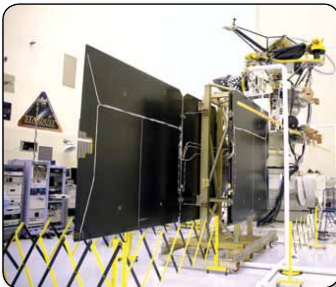
Inside Kennedy Space Center's Payload Hazardous Servicing Facility, an electromagnetic interference verification test is conducted on the solar arrays for the Mars Reconnaissance Orbiter (MRO) and an antenna simulator (yellow horizontal rod).
