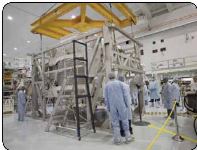
In the Space Station Processing Facility at NASA's Kennedy Space Center in Florida, an overhead crane lifts the Alpha Magnetic Spectrometer, or AMS, so it can be lifted onto a work stand and processed for launch.
