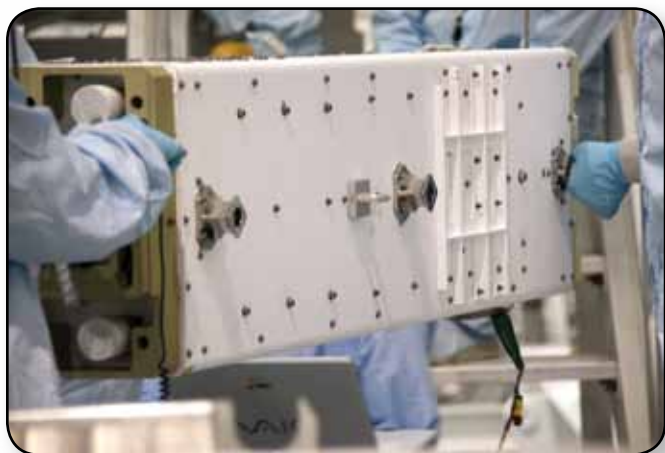
Technicians in Kennedy Space Center's Space Station Processing Facility prepare to install the EXPRESS Pallet Controller Avionics-4 to EXPRESS Logistics Carrier-4.
