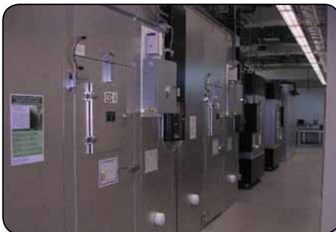
Kennedy Space Center's Controlled Environment Laboratory houses several controlled environment chambers that can be used to study plant growth for life support systems, preparing plants for spaceflight payloads, or testing under tightly controlled conditions.
