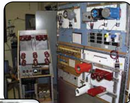
The hydrogen leak and fire detectors test stand enables Kennedy Space Center to perform advanced leak detection.
