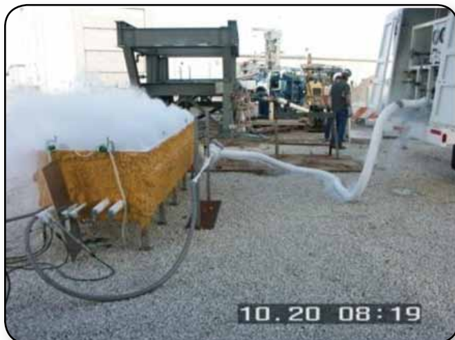
Ground support equipment designed at Kennedy Space Center is used to transfer cryogenic fluid. Condensation caused by the extremely cold fluid is visible in this image.
