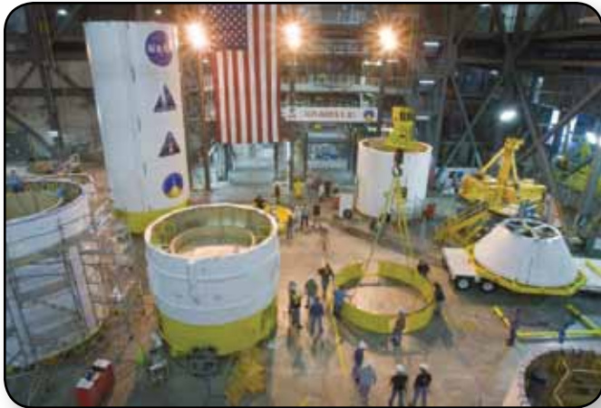
Various sections of the Ares I-X flight test vehicle are prepped and staged for integration inside Kennedy Space Center's Vehicle Assembly Building.
