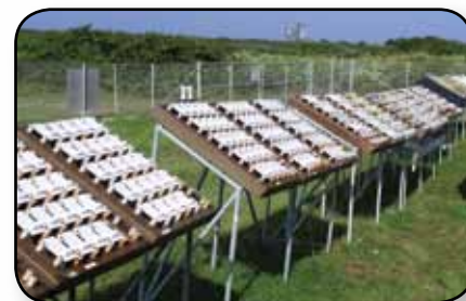
A close-up image of exposure racks used for research and testing at the Beach Corrosion Test Site.
