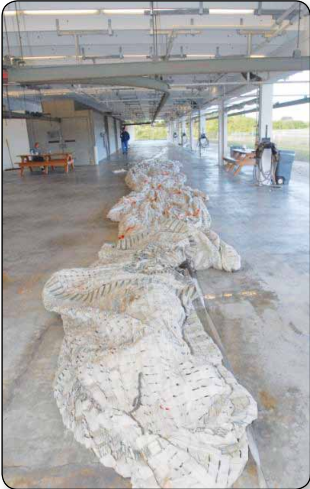
Parachutes recovered from sea after the launch of space shuttle Endeavour on the STS-126 mission are stretched out at the Parachute Refurbishment Facility to detangle them.
