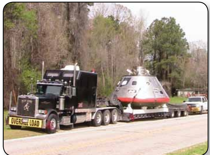
KSC teams planned and coordinated a demonstration of the truck transportation concept for the Orion crew module.
