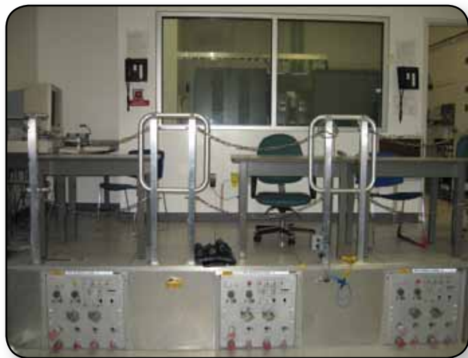
The PRCU provides a high-fidelity integration and testing environment by simulating the International Space Station interfaces.
