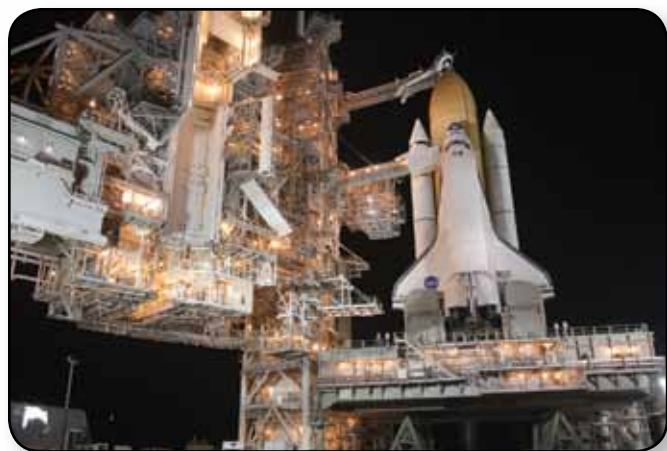
At Kennedy Space Center's Launch Pad 39A, space shuttle Discovery is visible following the retraction of the rotating service structure. The structure provides weather protection and access to the shuttle while it awaits liftoff on the pad.
