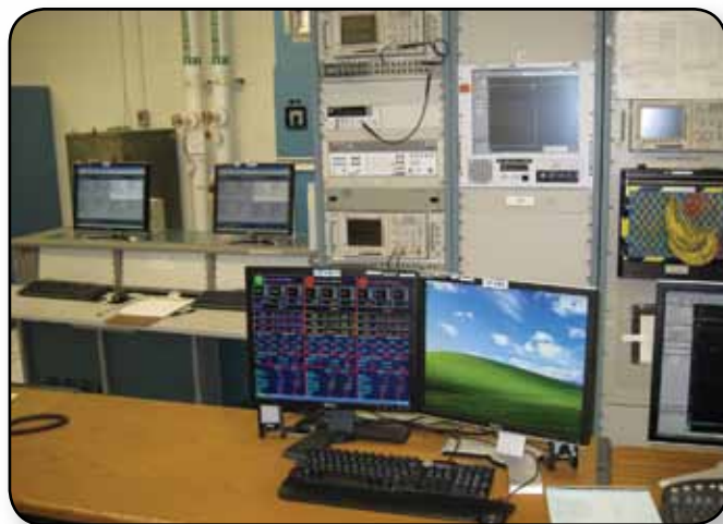
Components of Kennedy Space Center's Record and Playback Subsystem, including the Master Timing Unit, Dewetron client display and Dewetron recorders, are displayed.
