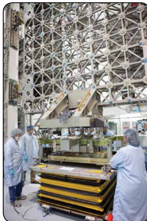
Workers performing a "fit check" of an EXPRESS Logistics Carrier to test electrical and mechanical attachment mechanisms.
