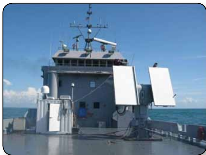
Kennedy Space Center utilizes one of the space shuttle solid rocket booster retrieval ships, Liberty Star, for X-band mobile radar.
