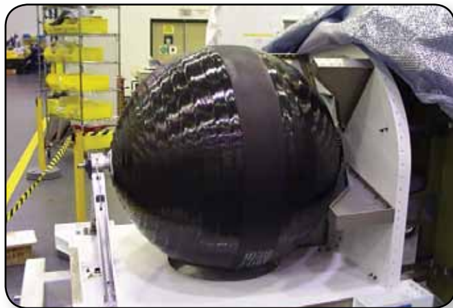
This composite overwrapped pressure vessel, which is used as a payload's high pressure gas tank, is an example of a tank that is serviced at Kennedy Space Center.
