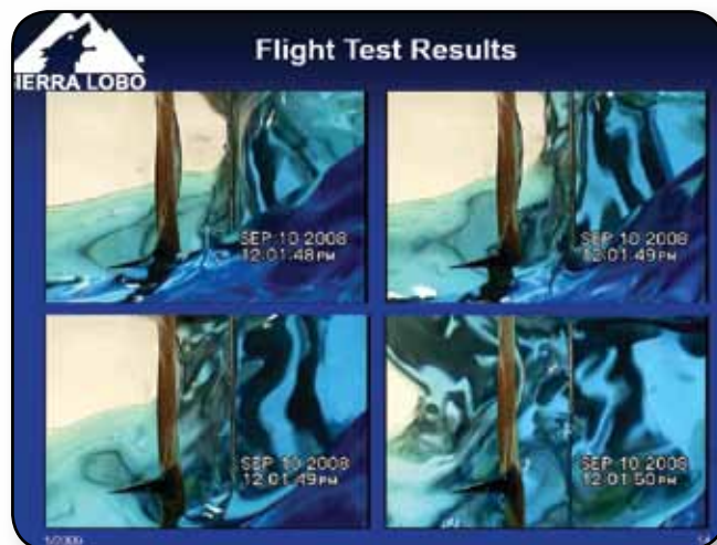
The CRYOTE tests demonstrate the feasibility of a liquid-sensing device designed for operation in microgravity environments.
