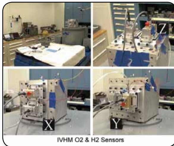
Hydrogen and oxygen point sensors are qualified at Kennedy Space Center.
