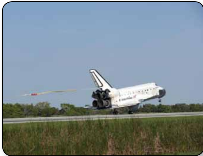
Space shuttle Discovery's 40-foot-diameter drag chute extends with the aid of a mortar-deployed pilot chute.
