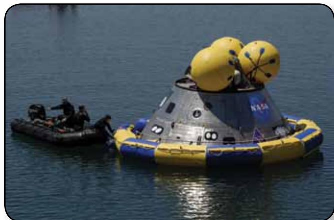
Members of the 920th Rescue Wing secure a flotation collar around a mock-up of the Orion crew exploration vehicle at the Trident Basin at Port Canaveral in Florida.
