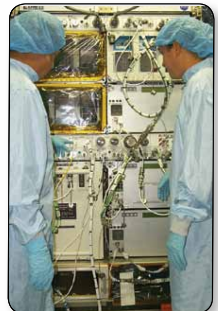
Technicians monitor the testing of an Expedite the Processing of Experiments to the Space Station (EXPRESS) rack.
