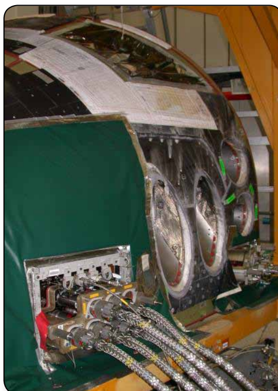
The interface connections for the Forward Reaction Control System (FRCS) thrusters of the orbiter uses hypergolic propellants.
