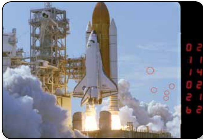
During foreign object debris (FOD) analysis of a space shuttle launch, the red circles indicates water ice was detected by image analysis.
