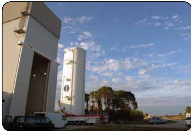
The payload canister containing the payload for space shuttle Endeavour's STS-126 mission backs away from the Canister Rotation Facility at Kennedy Space Center.
