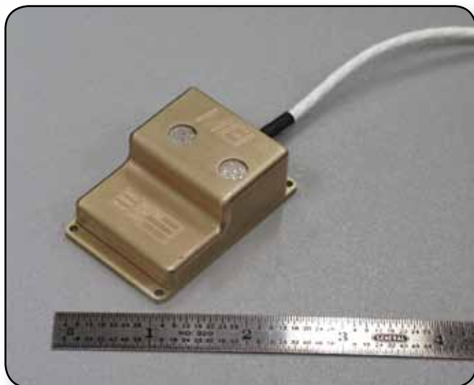
An image of the third-generation Hydrogen Point Sensor that monitored hydrogen concentrations in the aft section of the orbiter during space shuttle missions STS-95 and STS-96.
