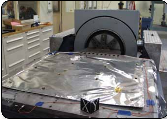
An electrostatic evaluation is performed on the space shuttle thermal control system multilayer blankets.
