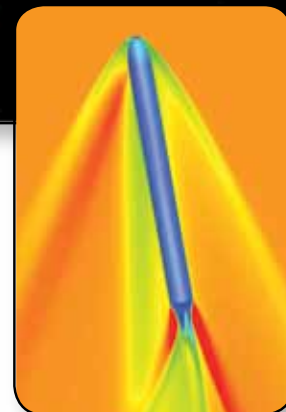
Mach contours and surface pressure coefficients for a blunted ogive-topped cylinder, Mach Number=2.5, Angle of Attack=10 degrees.
