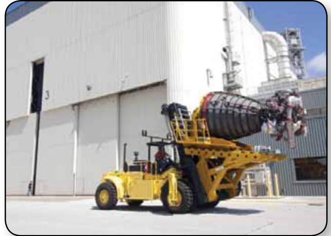
A space shuttle main engine is secured on a Hyster forklift as it is moved from the Space Shuttle Main Engine Processing Facility to Orbiter Processing Facility-3 at Kennedy Space Center.
