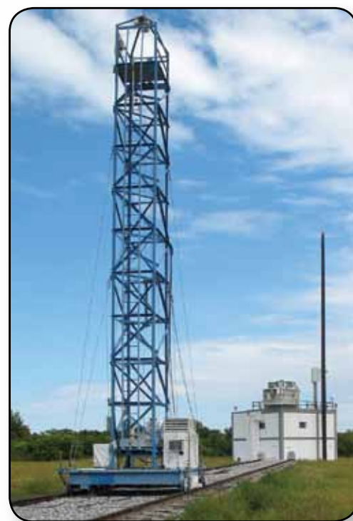
The adjustable source tower is positioned next to the Far Field Antenna Test Facility.
