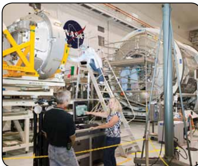
High-precision laser alignment ensures proper mating.
