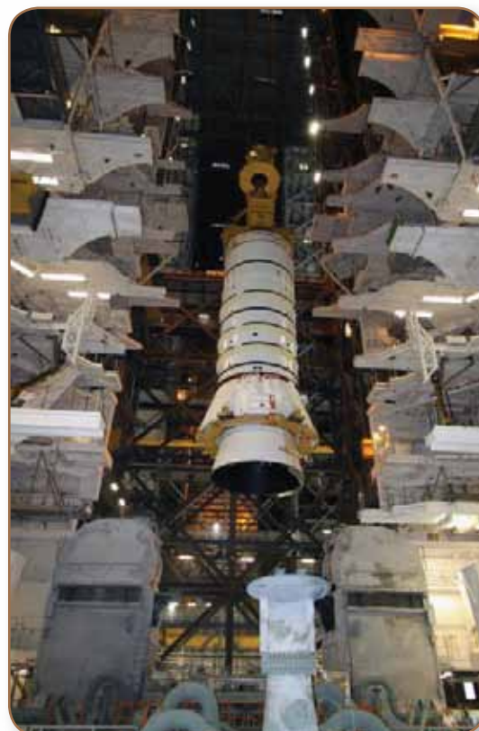
Workers carefully lift a solid rocket motor segment for the Ares I-X project.
