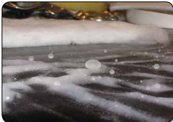
A close-up image of how hydrophobic aerogels are used in composites for low temperature applications at Kennedy Space Center.
