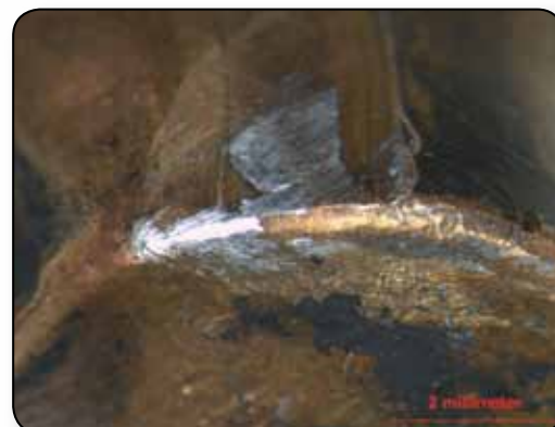
The bright markings on the base of the bullet are aluminum deposits from the window casing indicating that the bullet impacted tail first and sideways. This evidence indicates that the bullet was tumbling as it would after a ricochet.
