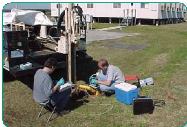
Environmental specialists collect depth specific groundwater samples using Direct Push Technology.
