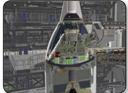
A simulated cutaway view shows the Orion spacecraft in the Vehicle Assembly Building.
