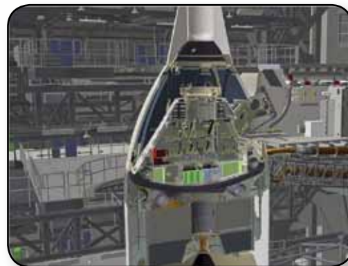
A simulated cutaway view shows the Orion spacecraft in the Vehicle Assembly Building.
