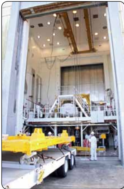
At the Hypergolic Maintenance Facility at NASA's Kennedy Space Center in Florida, preparations are under way to move the Forward Reaction Control System, or FRCS, for space shuttle Discovery to Orbiter Processing Facility Bay 3.
