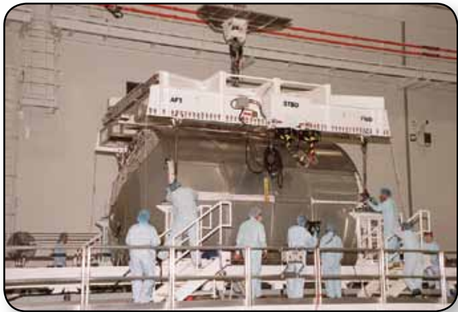
The multi-purpose logistics module Leonardo rests on the weight and balance scale in Kennedy Space Center's Space Station Processing Facility.
