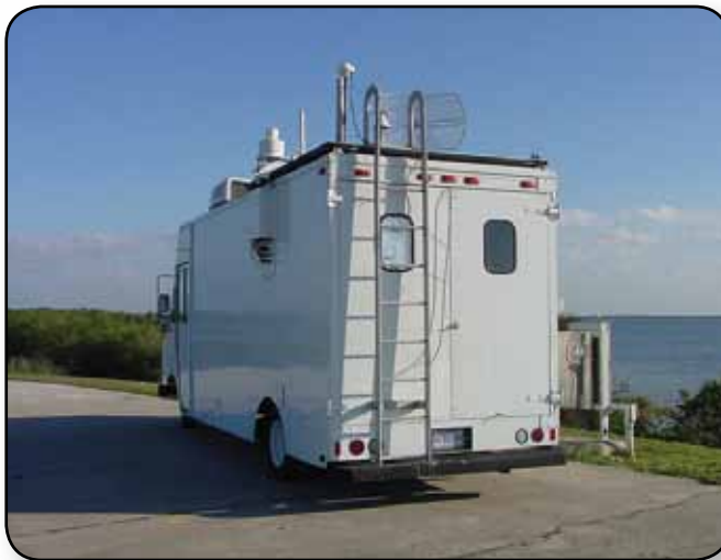
The mobile electromagnetic van is a portable environment surveillance system used by Kennedy Space Center to detect electromagnetic interference.
