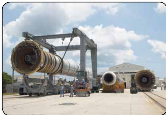
At the Solid Rocket Booster Disassembly Facility at Hangar AF at Cape Canaveral Air Force Station, a mobile gantry crane lifts one of the solid rocket boosters used during space shuttle Atlantis' STS-132 launch.
