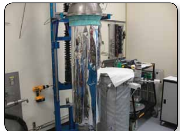
A multilayer insulation system is prepared at Kennedy Space Center and readied for installation in a guarded liquid nitrogen calorimeter.
