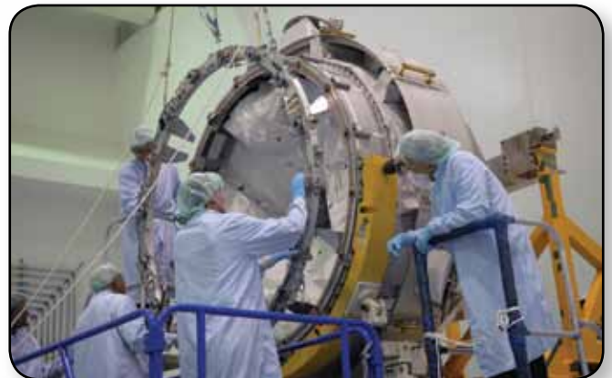
Technicians attach a common berthing mechanism onto the cupola, a seven-window module that was delivered to the International Space Station during the STS-130 mission in February 2010.
