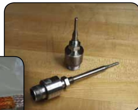
Cryogenic temperature probes are used for cryogenic operations at Kennedy Space Center.
