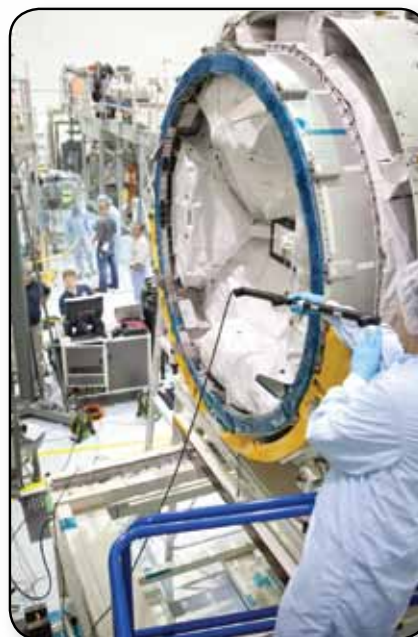
Inside Kennedy Space Center's Space Station Processing Facility, a technician takes a precise measurement of a payload that will be delivered to the International Space Station.
