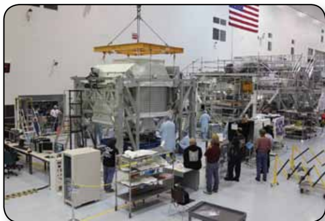
International partners install the Passive Attach System (PAS) to the Alpha Magnetic Spectrometer (AMS). The scheduling of resources to support multiple customers' needs is carefully coordinated by Kennedy Space Center and spacecraft customer support personnel.
