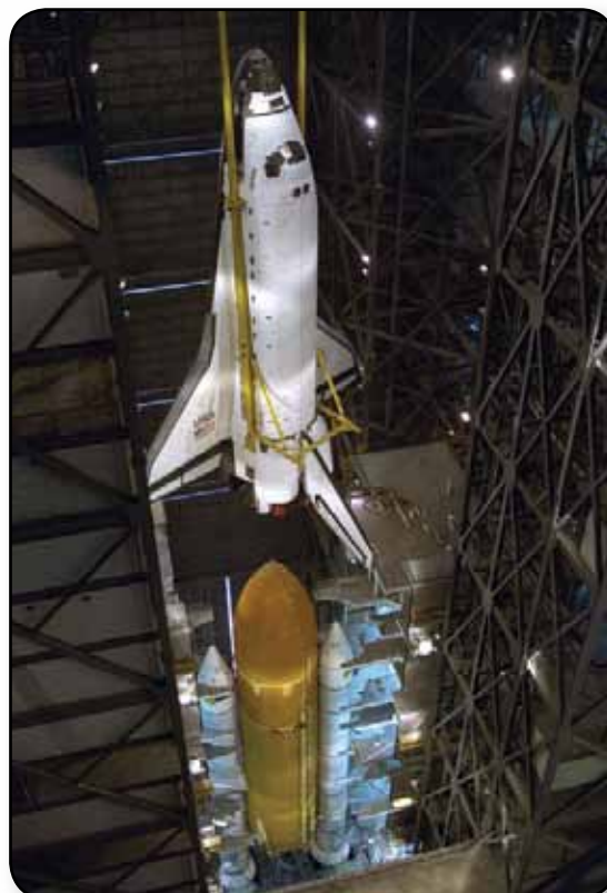
A vantage point from high above in Kennedy Space Center's Vehicle Assembly Building yields a dramatic view of an orbiter being mated to its stack.
