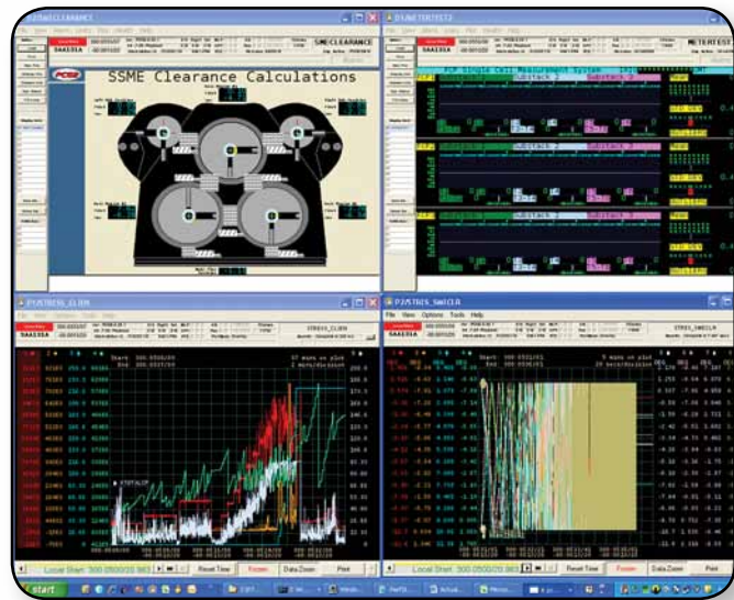
A real-time monitor display of the telemetry monitoring system shows a sample of space shuttle main engine gimbaling data.
