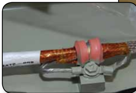
This close-up shows the final splicing completed on the wiring between space shuttle Atlantis' external tank and the engine cutoff (ECO) sensor system. Cryogenic shielding is installed around the wiring.
