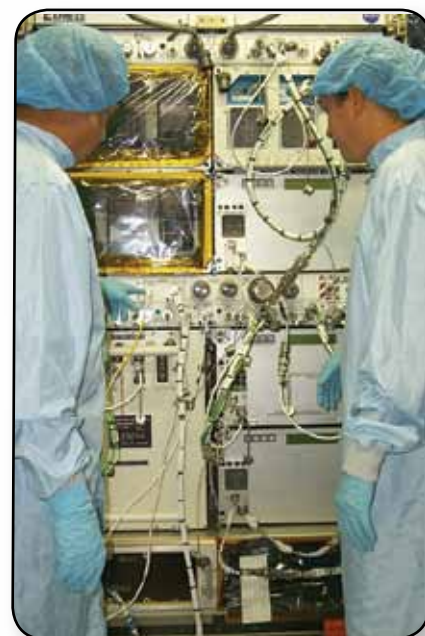
Technicians monitor the testing of an Expedite the Processing of Experiments to the Space Station (EXPRESS) rack.
