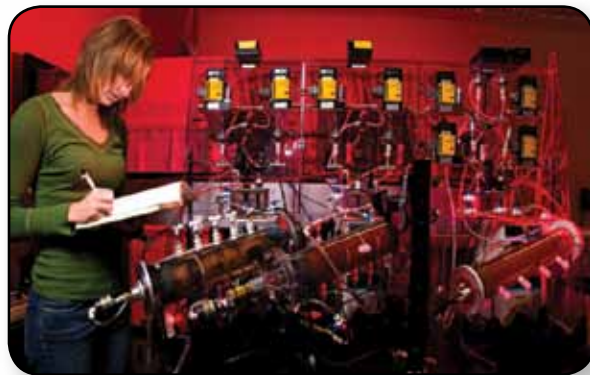
Kennedy Space Center's wastewater bioreactors purify wastewater by utilizing fiber membranes and microbial communities that convert ammonium nitrogen (e.g., from urine) into nitrate, or N2 gas.
