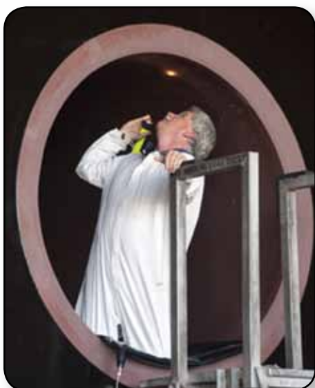
A technician inspects the inner core of a solid rocket motor.
