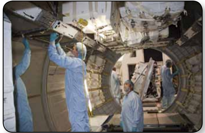
In Kennedy Space Center's Space Station Processing Facility, technicians work to unload returning cargo from the International Space Station stored inside the multi-purpose logistics module Leonardo.
