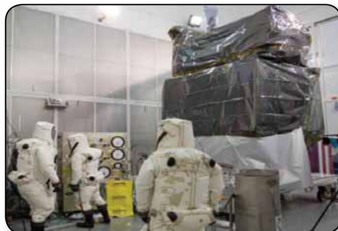
Technicians at Kennedy Space Center perform hypergolic servicing of the Solar Dynamics Observatory spacecraft.
