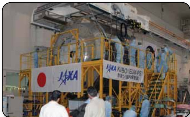
In the Space Station Processing Facility, workers attach a crane to the Experiment Logistics Module Pressurized Section, or ELM-PS, of the Japanese Experiment Module, called Kibo, so that Japan Aerospace Exploration Agency workers can begin processing work.
