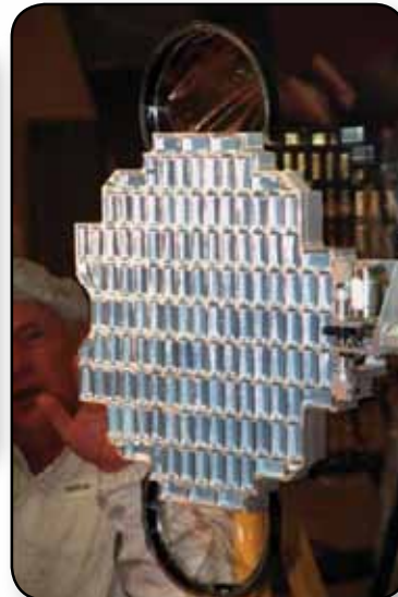
In Kennedy Space Center's Payload Hazardous Servicing Facility, the aerogel grid is deployed from the Stardust Sample Return Capsule (SRC). The unique properties of aerogel allowed the Stardust capsule to capture comet particles
