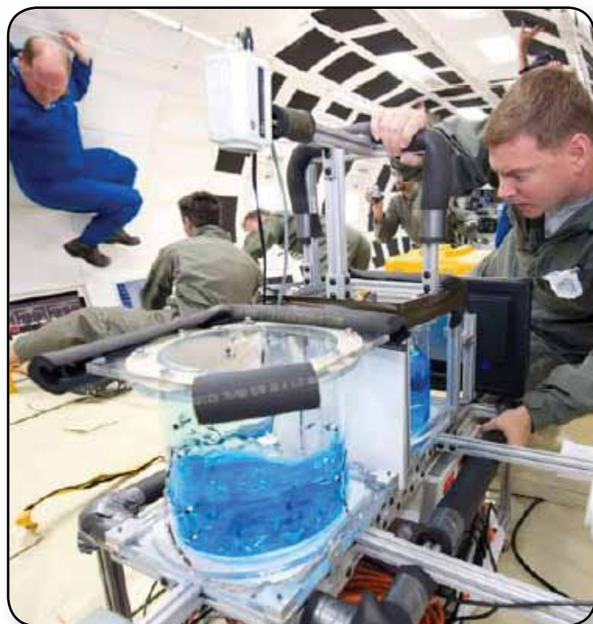
The Cryogenic Orbital Testbed (CRYOTE) is studied on board a reduced gravity aircraft. The thermal group partnered with universities and industry in developing CRYOTE.
