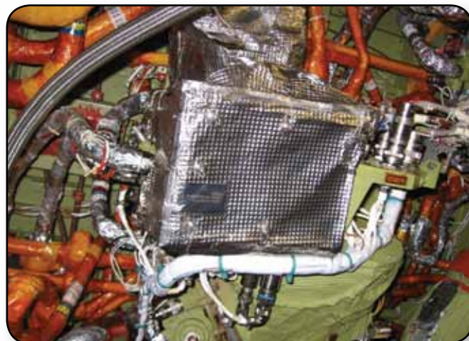
An assessment was performed to evaluate the risks of an electrostatic discharge from ungrounded metallic thermal blankets located in the aft compartment of the orbiter.
