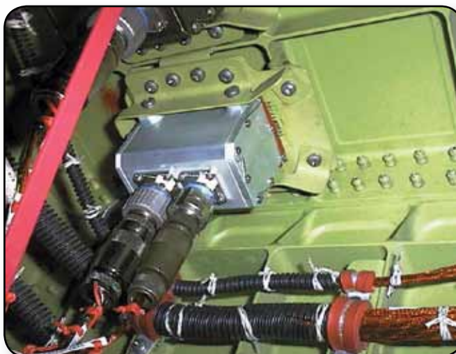
A hydrogen point sensor is mounted in the aft section of a space shuttle.
