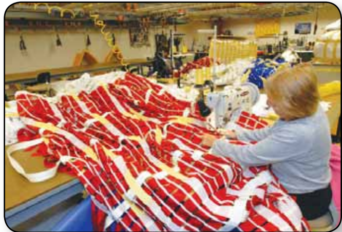
In the Parachute Refurbishment Facility, workers repair the parachutes recovered from sea after the launch of space shuttle Endeavour on the STS-126 mission.
