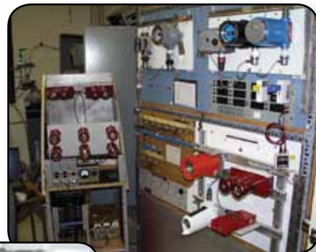
The hydrogen leak and fire detectors test stand enables Kennedy Space Center to perform advanced leak detection.
