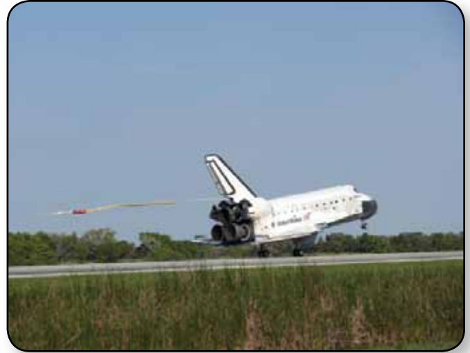
Space shuttle Discovery's 40-foot-diameter drag chute extends with the aid of a mortar-deployed pilot chute.
