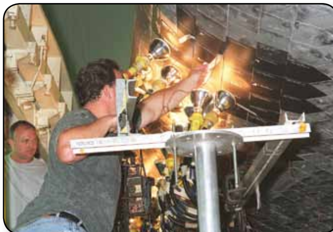
A technician points to some of the tiles on orbiter Atlantis that are being dried by clusters of 200-to-300 watt heat lamps.
