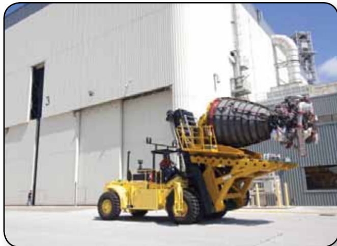
A space shuttle main engine is secured on a Hyster forklift as it is moved from the Space Shuttle Main Engine Processing Facility to Orbiter Processing Facility-3 at Kennedy Space Center.
