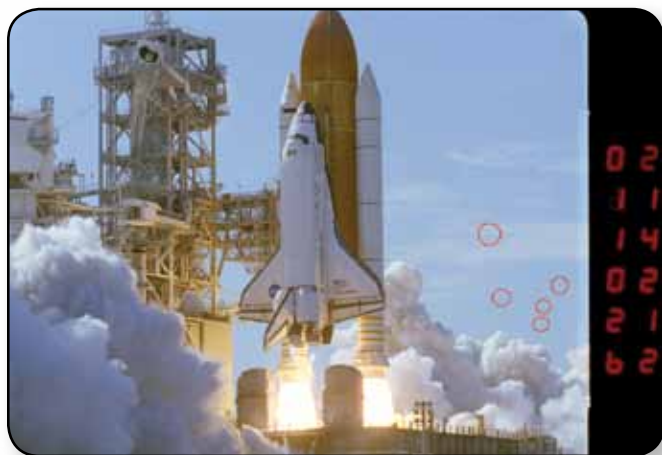
During foreign object debris (FOD) analysis of a space shuttle launch, the red circles indicates water ice was detected by image analysis.
