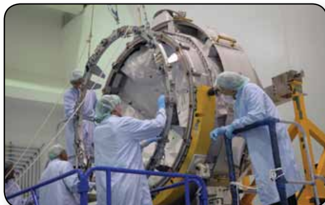
Technicians attach a common berthing mechanism onto the cupola, a seven-window module that was delivered to the International Space Station during the STS-130 mission in February 2010.
