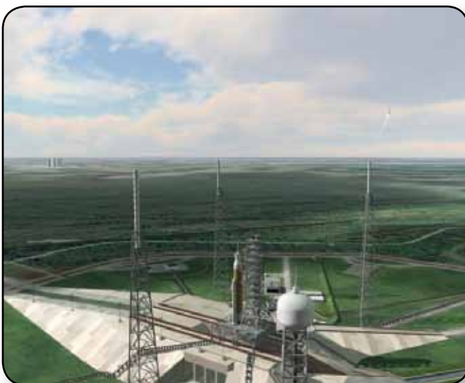
An artist's rendering of a shuttle-derived heavy-lift launch vehicle is shown on Launch Pad 39B as it is being readied for launch with a multipurpose crew vehicle. This is just one concept being evaluated for NASA's new space launch system.
