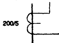
Figure 9-14. Current Transformer Ratio
