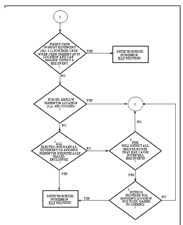
$<sup>^3</sup>$  Aviorics refers to any electrical equipment or components other than power/data connectors, cables, lines, or wires  $_2$  (e.g., card mounted electronic components). Electro-mechanical equipment refers to any motors, pumps, etc.
