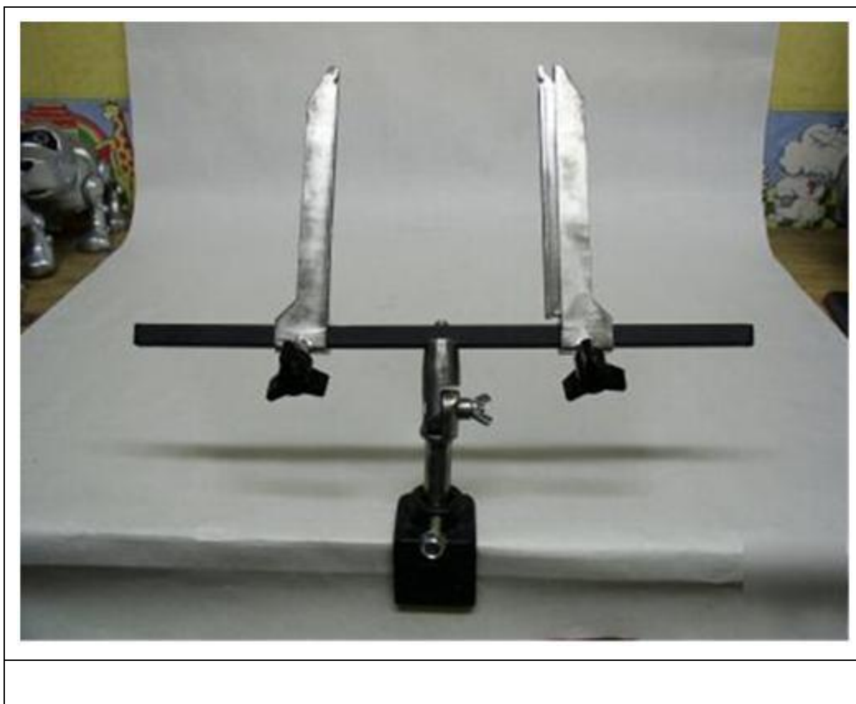
Figure 8-2 Board Clamps to Hold DUT Circuit Board In Front Of NSRL Beam
