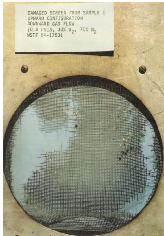
Figure 10. Damaged Aluminum Vent Screen from Airflow Tests
