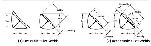
Note: Convexity of a weld or individual surface bead with dimension Width shall not exceed the value of the following table.
