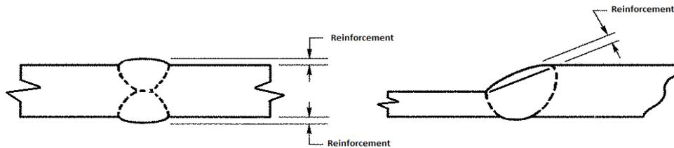
**(4) Acceptable Groove Weld Profiles in Butt Welds**
