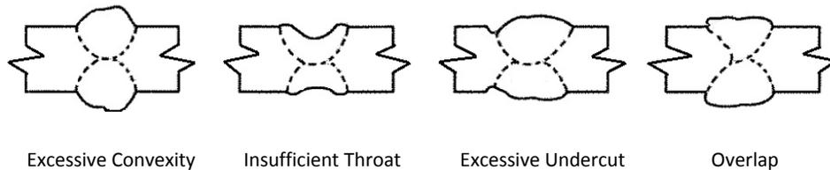
**(5) Unacceptable Groove Weld Profiles in Butt Joints**
