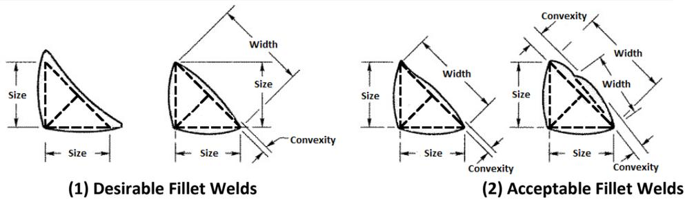
Note: Convexity of a weld or individual surface bead with dimension Width shall not exceed the value of the following table.
