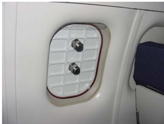
Figure 6B. Dedicated Overboard Vent Ports
