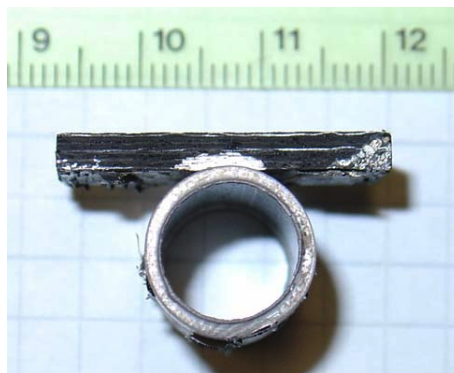
Figure 5.3-4. C/C to Ti brazing trials.
