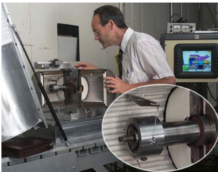
Figure 5.3-2. High-Pressure Bearing Test Rig.
