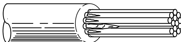
Figure 3.13-81 Unacceptable Mechanically Stripped, Nicked and/or Severed Strands.
