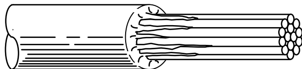
Figure 3.13-76 Unacceptable Thermally Stripped, Insulation with Icicles.
