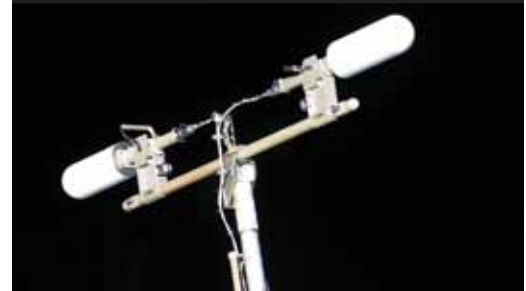
UHF antenna on the P1 Truss.
