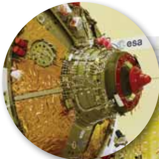
Russian-built probe and drogue docking system.
