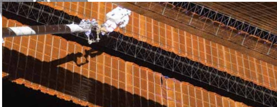
Astronaut Scott Parazynski, anchored to the Articulating Portable Foot Restraint (APFR) on the Orbiter Boom Sensor System (OBSS), assesses repair work on the P6 4B Solar Array Wing (SAW) as the array is deployed during an extravehicular activity (EVA).
