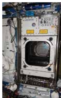
Provides a facility for Earth science research using the Destiny science window on the ISS.
