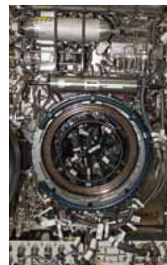
Used to perform sustained, systematic combustion experiments in microgravity.
