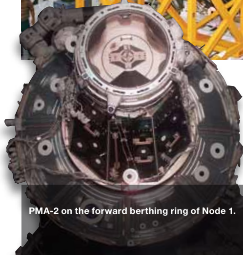
PMA structure shows a series of offset aluminum cylinders.
