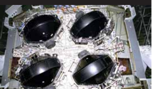
Control Moment Gyroscope gimbals used for orienting the ISS.
