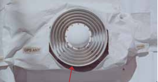
GPS antenna on S0 Truss.
