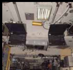
The Tissue Equivalent Proportional Counter (TEPC) measures radiation dose and dose equivalents.
