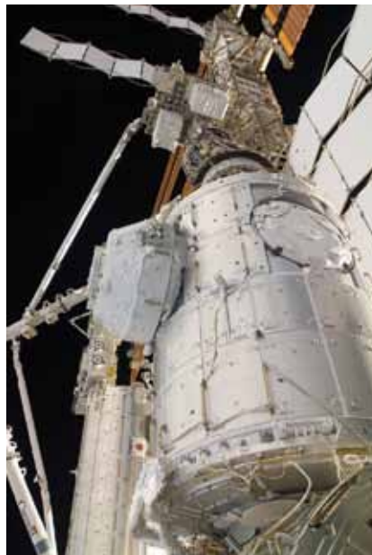
In the grasp of the Canadarm2, the Pressurized Mating Adapter 3 (PMA-3) is relocated from the Harmony node to the open port on the end of the newly installed Tranquility node.
