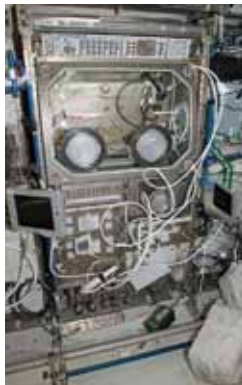
Provides a safe containment environment for research with liquids, combustion, and hazardous materials.
