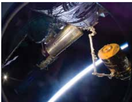
Canadarm2 unberths the HTV in preparation for its release from the ISS.
