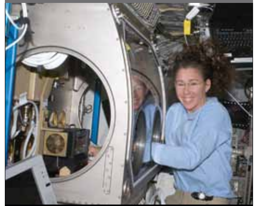
Astronaut works with the Smoke Point In Co-flow Experiment in the Microgravity Sciences Glovebox (MSG) during Expedition 18.
