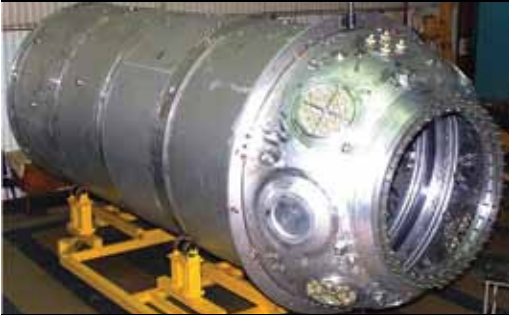
MRM1 Flight Article is manufactured from the pressurized compartment of the Science Power Platform (SPP) Dynamic Test Article.
