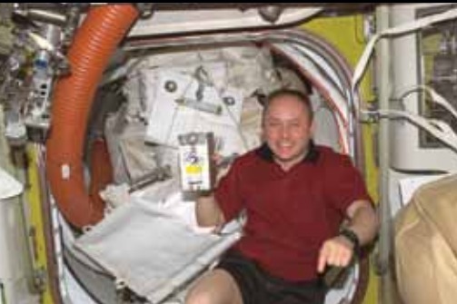
Crewmember Mike Fincke holds an RPCM in the Quest Airlock. It was later used to replace an RPCM on the S0 Truss.
