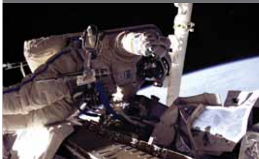
Crewmember Mike Fincke replaces the Remote Power Controller Module (RPCM) on the S0 Truss.
