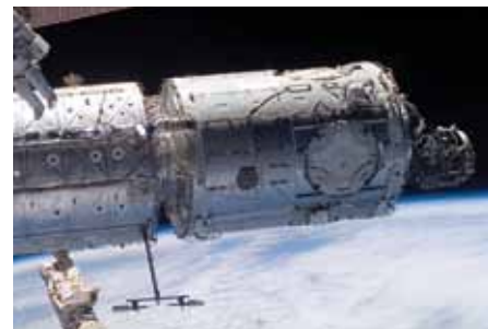
Node 2 after its installation during STS-120.
