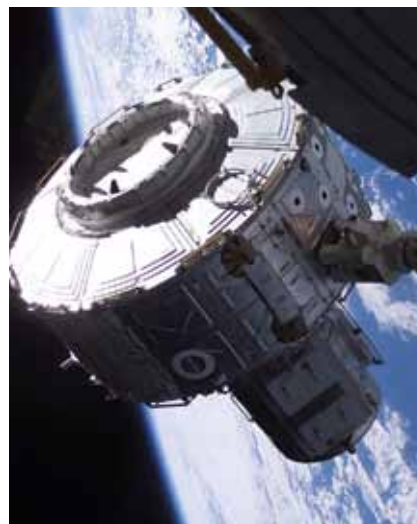
Space Shuttle mission STS-104 berths Quest to the starboard side of Node 1 in July 2001.
