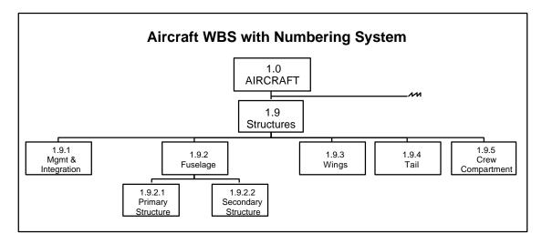
Normally, NASA will control only to the top three levels of the PWBS. The lower levels are controlled by contractors. Complete numbering system standardization and uniformity may not be possible since contractor coding systems vary from contractor to contractor. When possible, contractors should follow the PWBS numbering system in use.
