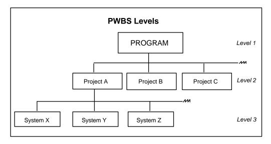
There are numerous terms used to define succeeding levels of the PWBS below the subsystem level. Some examples are equipment, assembly, subassembly, component, and part. The choice of which to use is made by project management.
