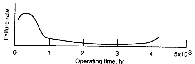
Figure 6-14.—Failure-rate characteristics of commercial jet electronic subsystem.
