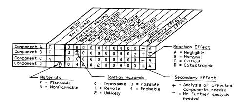
Figure 2 Oxygen Hazards Analysis Chart.
