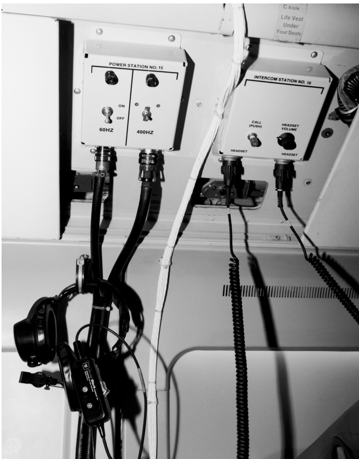
Figure 6-1. Typical power and intercom station in cabin.
