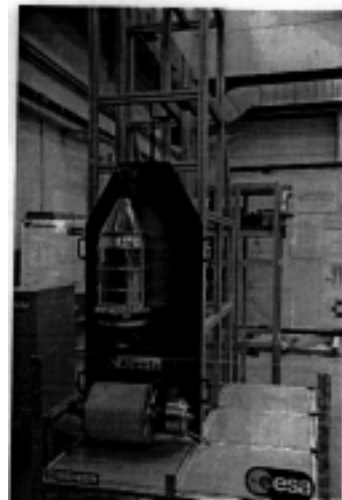
Figure 1. Expendable tether mechanism breadboard model
