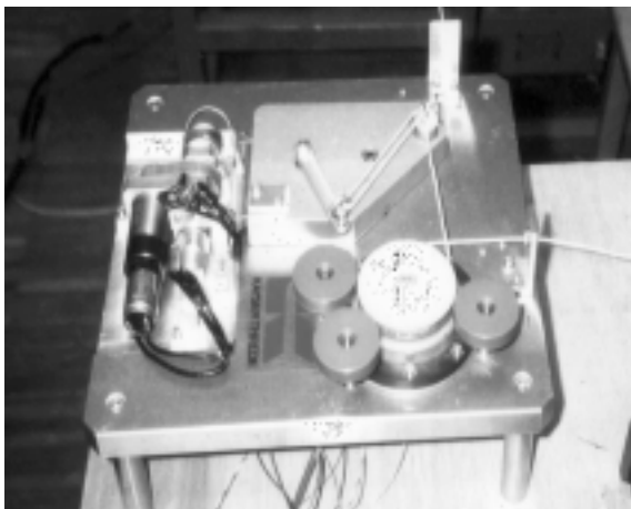
Figure 1. Breadboard model of tether deployer
