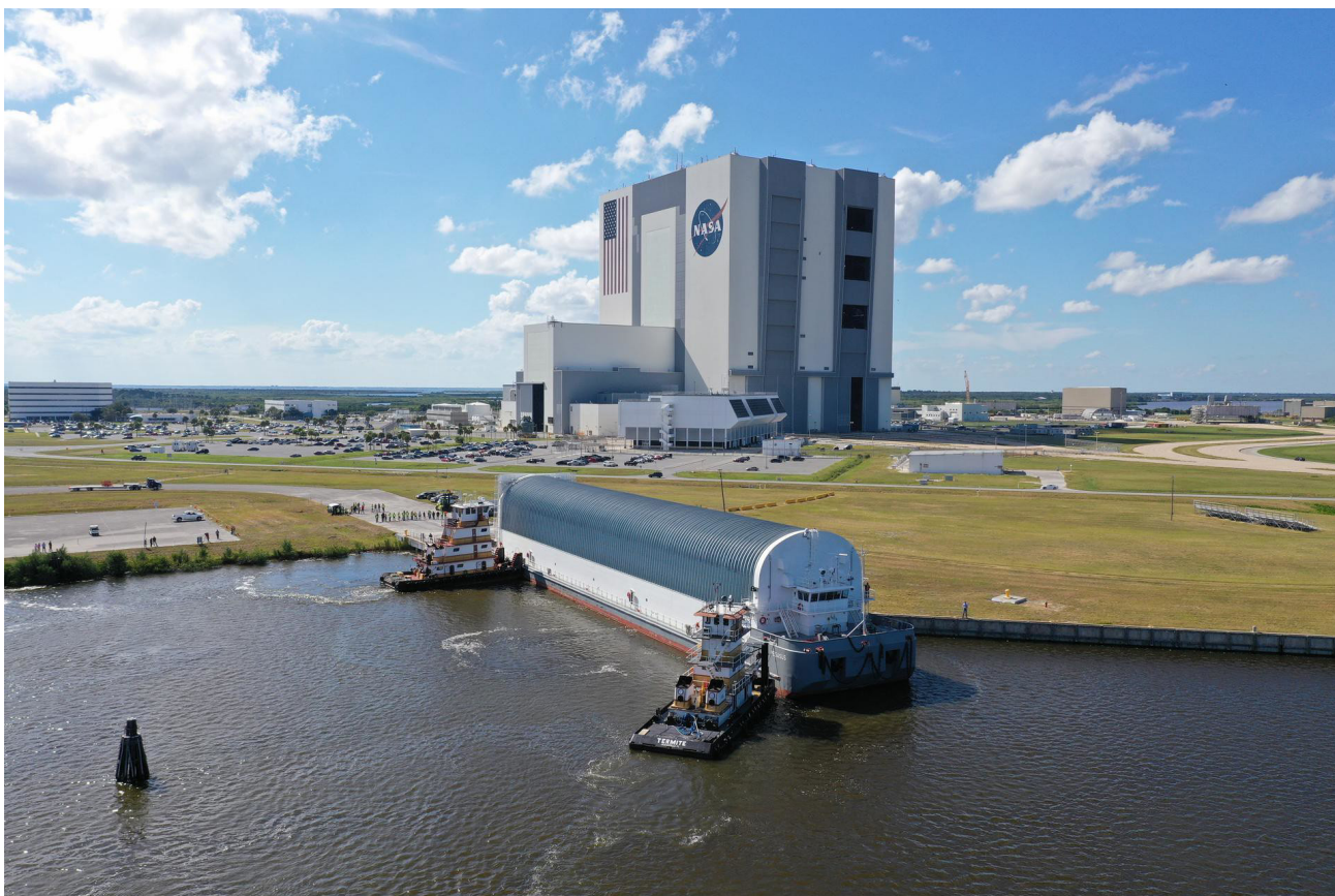
Space Launch System Mock Up arrives at Kennedy for Testing. NASA's Pegasus Barge arrived at the Launch Complex 39 turn basin wharf at Kennedy Space Center in Florida to make its first delivery to Kennedy in support of the agency's Artemis missions. The upgraded 310-foot-long barge arrived September 27, 2019, ferrying the 212-foot-long Space Launch System rocket core stage pathfinder. Weighing in at 228,000 pounds, the Pathfinder is a full-scale mock-up of the rocket's core stage and will be used to validate ground support equipment and demonstrate it can be integrated with Kennedy facilities.
