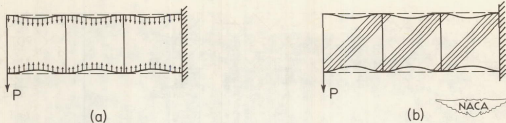
Figure 5.— Secondary actions in diagonal-tension beams.
