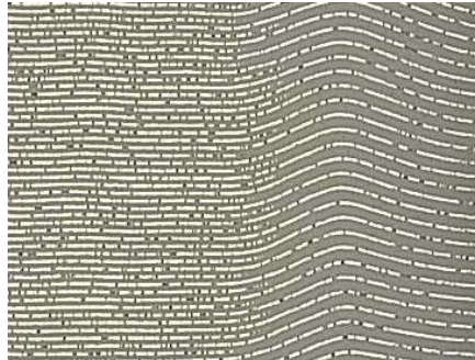
Figure 2 Acceptable undulation in electrode/dielectric layers
