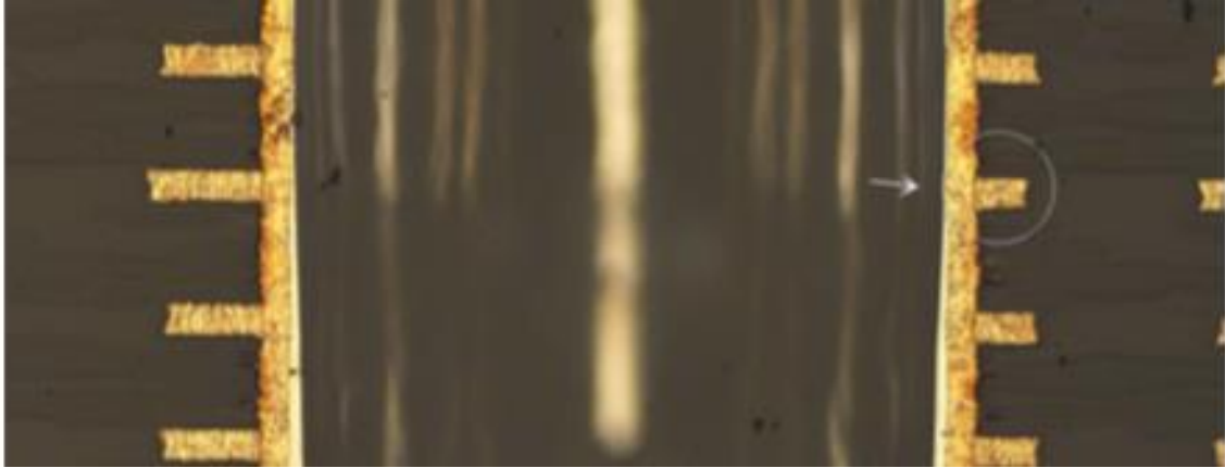
Figure A1: Plated throughhole in microsection
