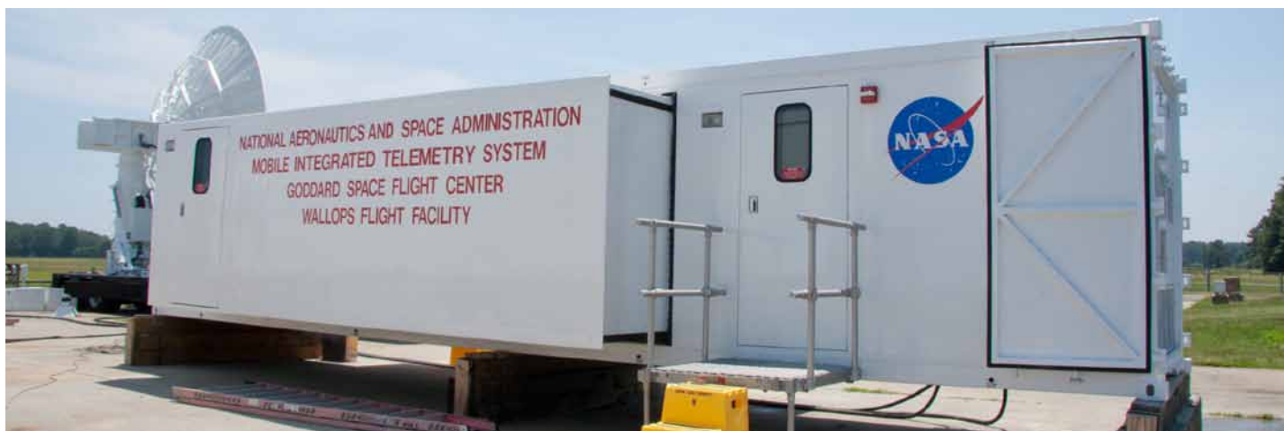
Figure 3-26. Mobile Integrated Telemetry Systems (MITS) Van
