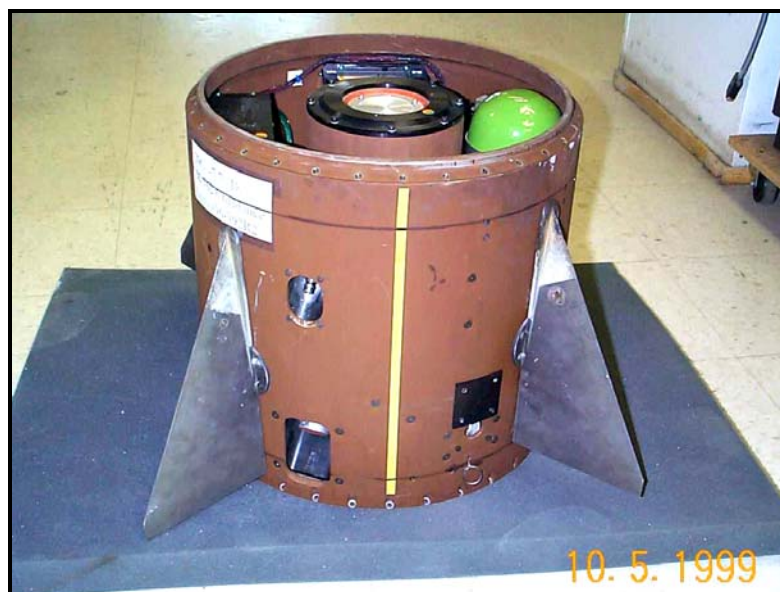
Figure 3.3.1-1b: S-19 Boost Guidance System
