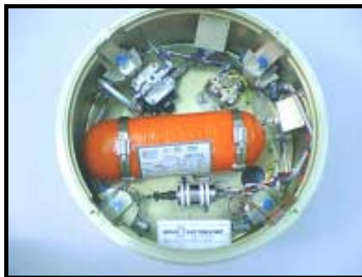
Figure I.4-1: Pneumatic subsystem, rate sensor, battery
