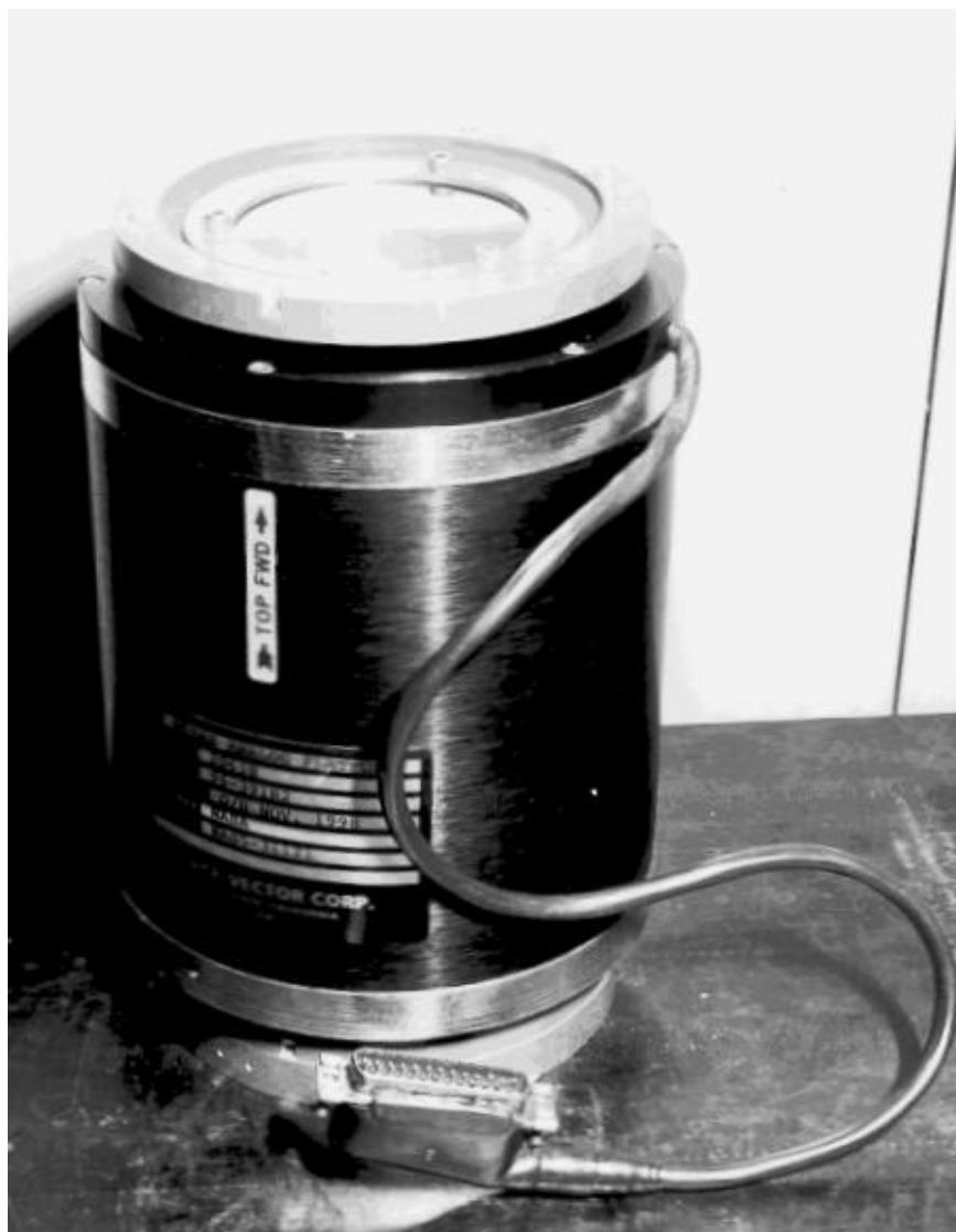
Figure 5-3. MIDAS Attitude Sensor
