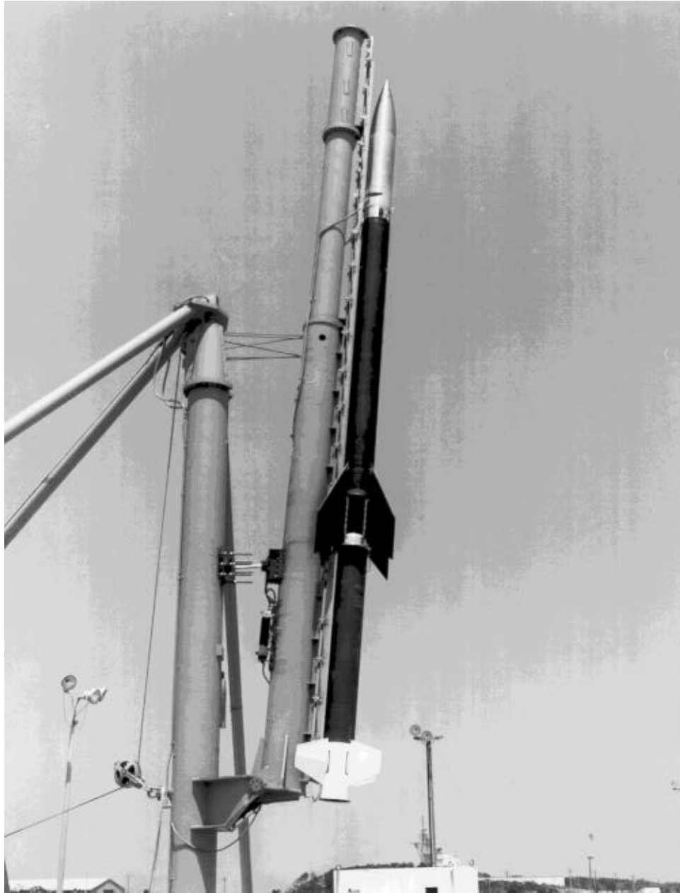
Figure E-6 Nike-Black Brant VC Launch Vehicle
