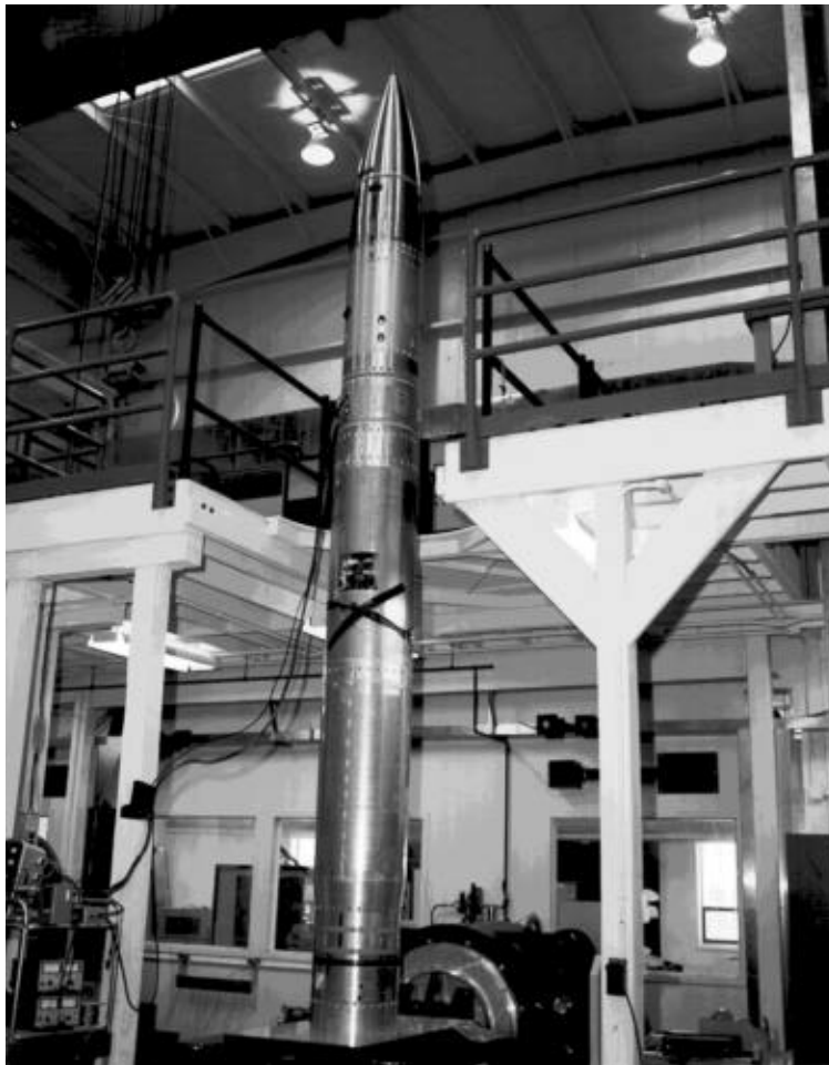
Figure 11-6. Astrophysics Payload (36.022) undergoing Lateral Vibration Testing
