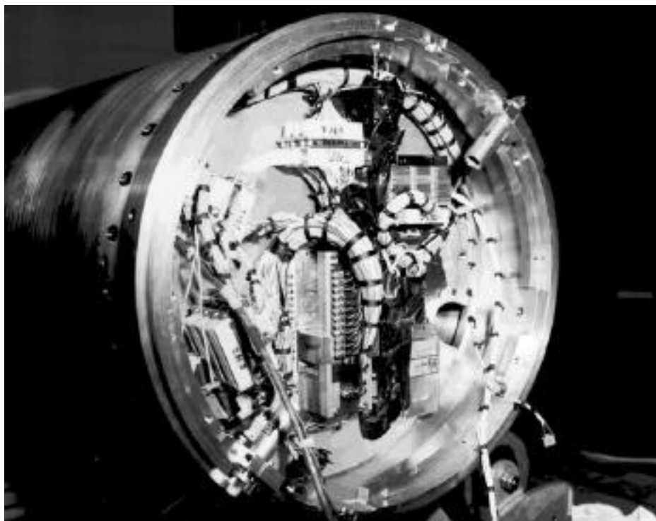
Figure 5-2. Typical WFF-93 PCM Encoder
