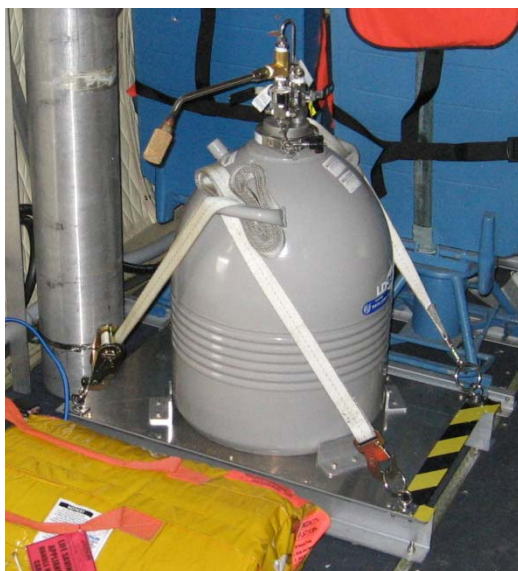
Figure 4-10. Typical pallet style installation
