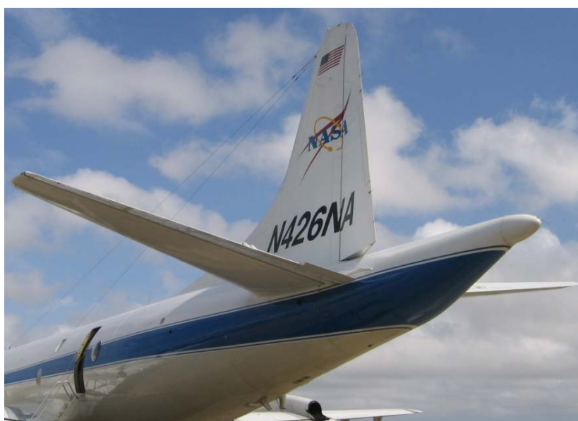
Figure 4-29. Nose radome and tailcone experimenter ports
