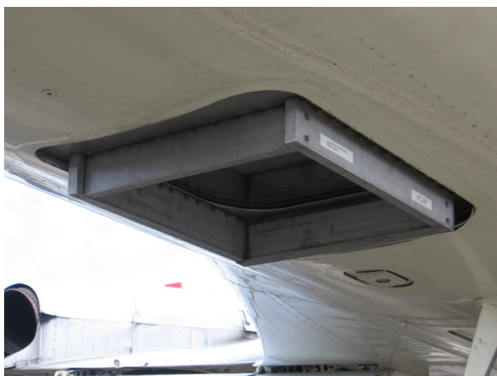
Figure 4-22. Nadir #2 port (with custom port plug installed)
