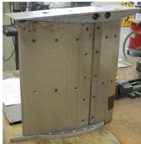
Figure 4-11. Existing wingtip pylon
