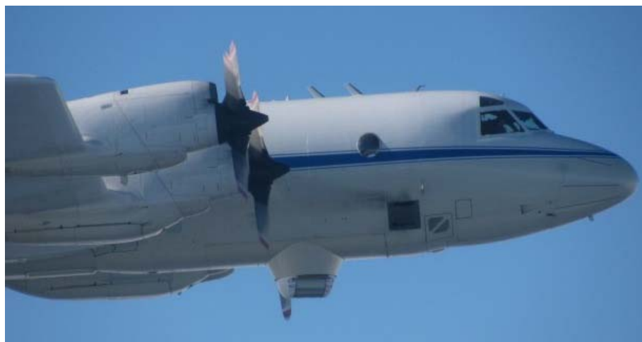
Figure 4-33. Custom bomb bay modification for the AESMIR installation
