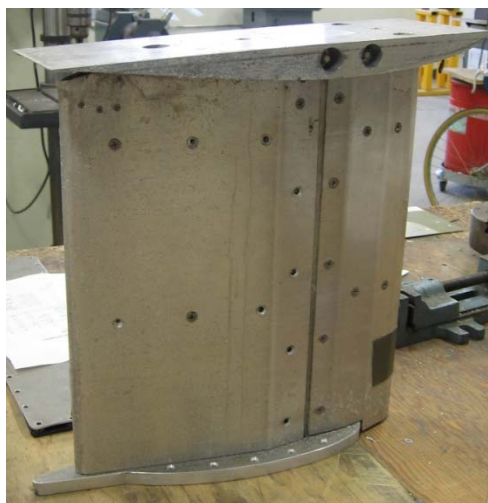
Figure 4-11. Existing wingtip pylon
