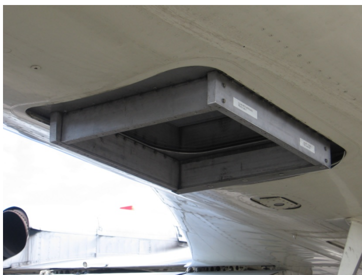
Figure 4-22. Nadir #2 port (with custom port plug installed)
