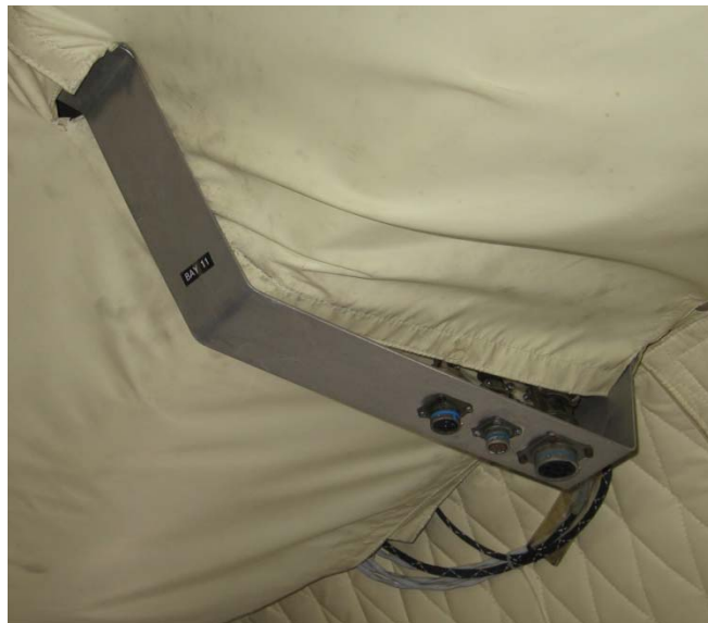
Figure 4-15. Typical power and intercom station in cabin
