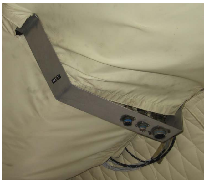
Figure 4-15. Typical power and intercom station in cabin
