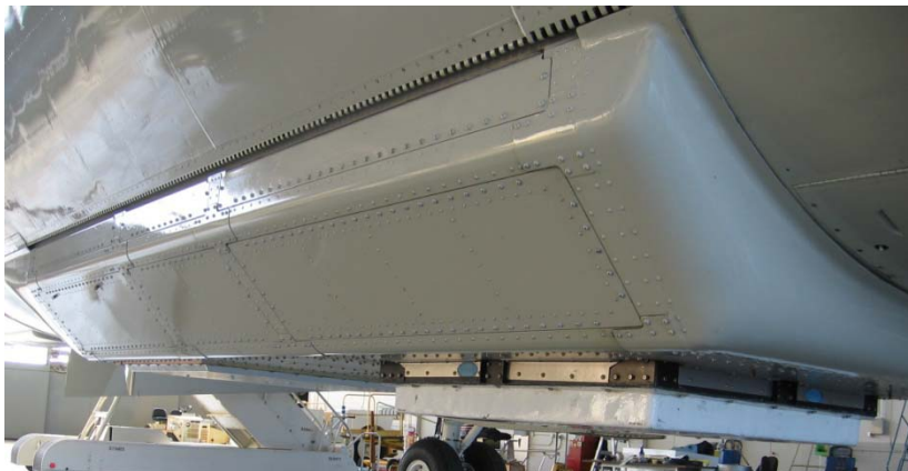
Figure 4-26. Bomb bay experimenter ports
