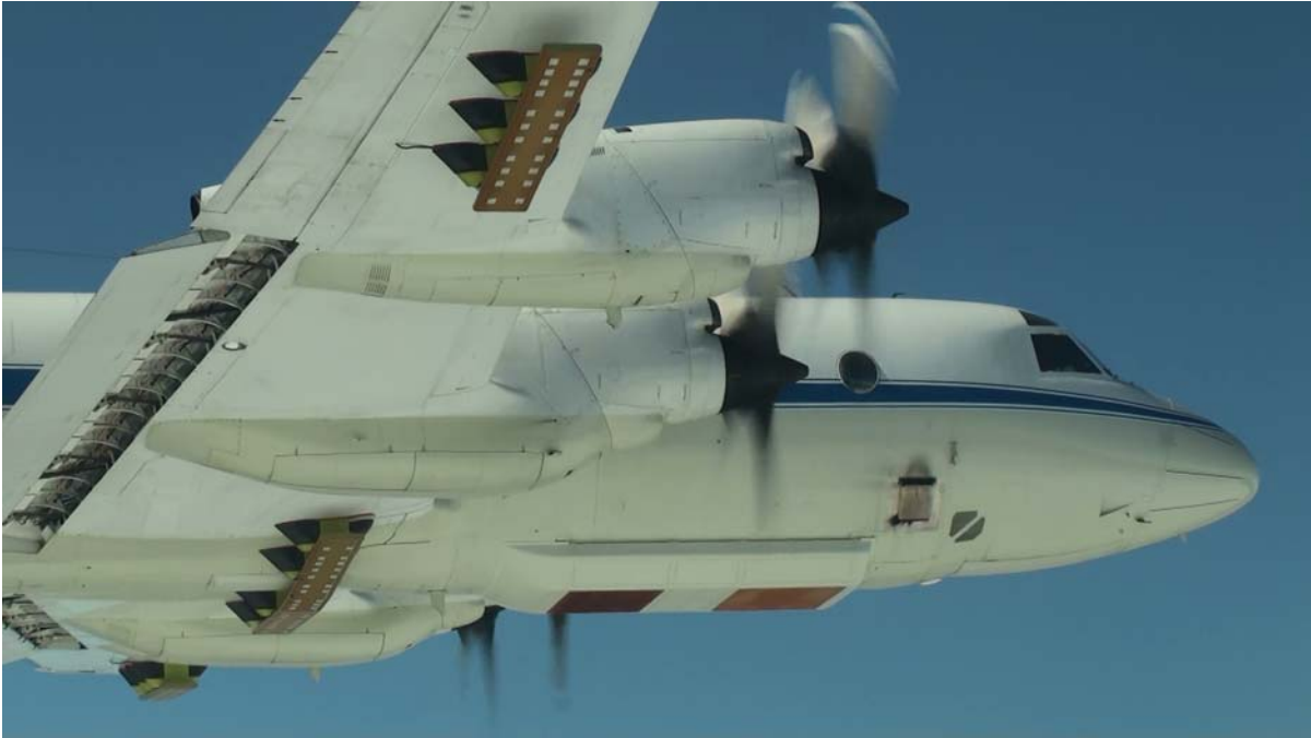
Figure 4-12. Custom under wing installation for KU MCoRDS antenna array
