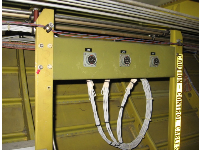
Figure 4-16. Power station below the cabin floor
