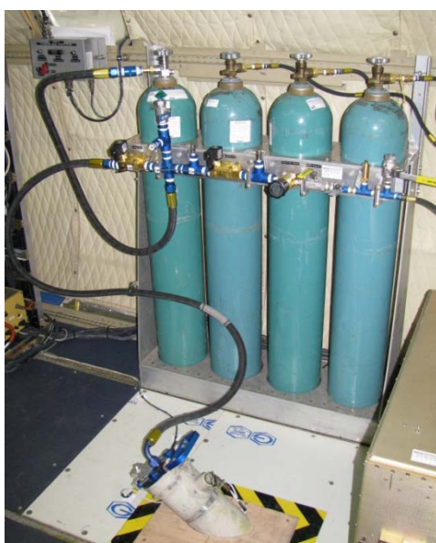
Figure 4-31. PSLT pressurized sonobuoy deployment installation
