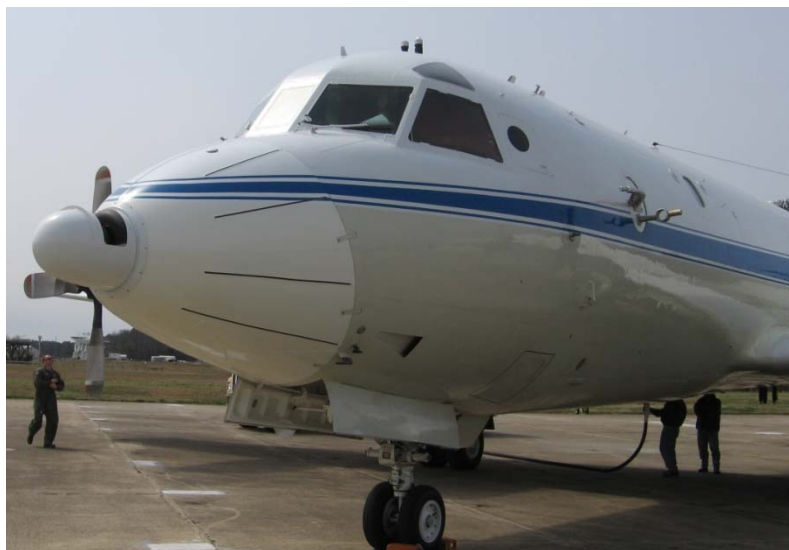
Figure 4-32. Custom nose radome modification for CAR installation
