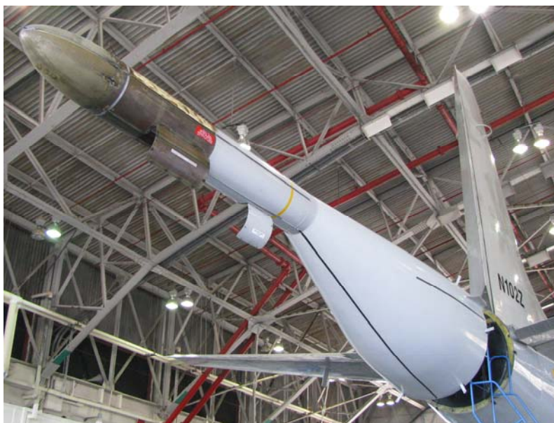
Figure 4-30. Tailcone with MAD boom extension
