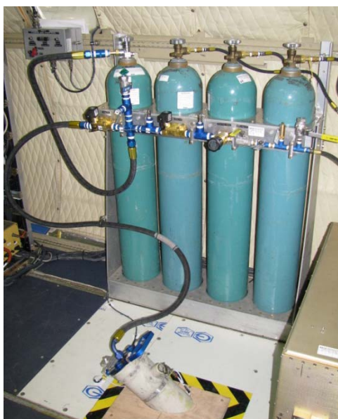
Figure 4-31. PSLT pressurized sonobuoy deployment installation
