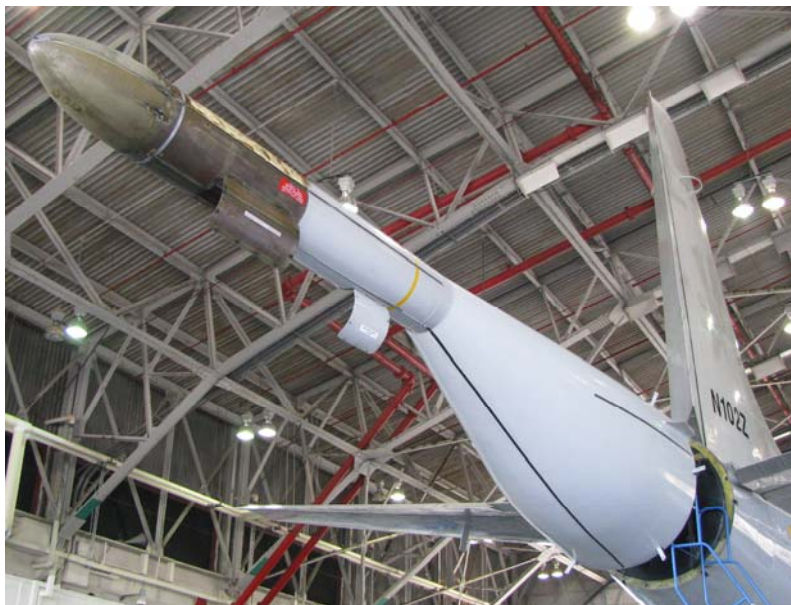
Figure 4-30. Tailcone with MAD boom extension
