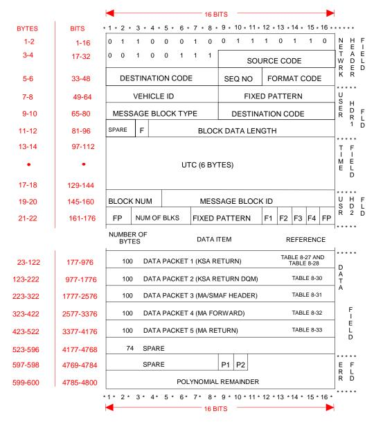
Note: Consists of up to three 4800-bit blocks, (block two).
