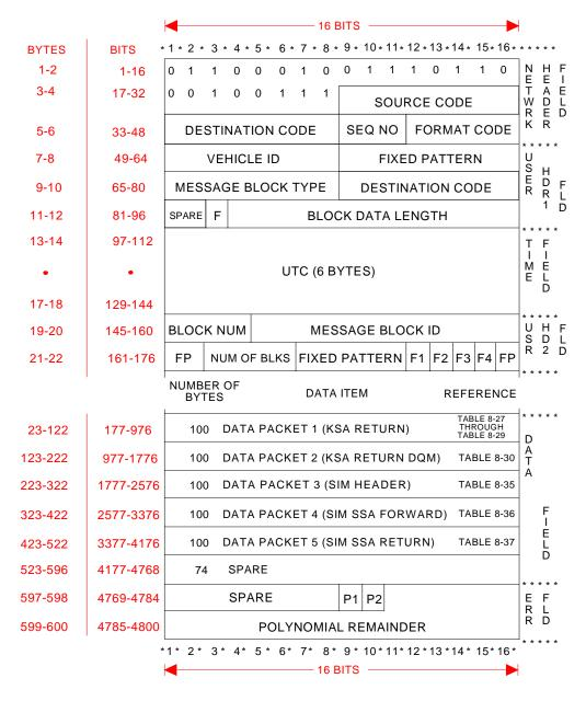
Note: Consists of up to three 4800-bit blocks, (block two).
