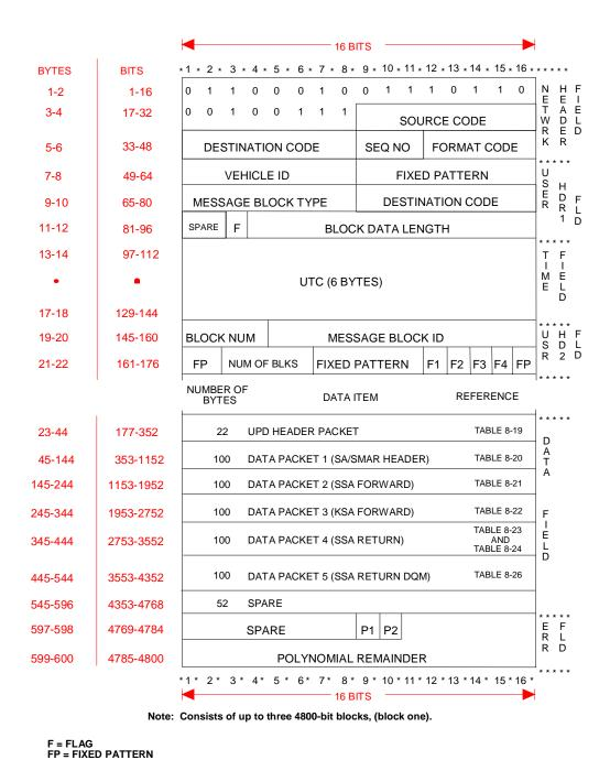
Figure 8-1. Example of Message Packing for SSA/KSA/MA (Forward/Return) and Simulation UPD - Nascom 4800-bit block protocol (1 of 3)
