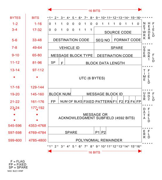
Figure 4-1. Nascom 4800-bit Block Format (MOC)
