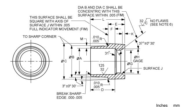
FIGURE 1. Ferrule, brazing, tube fitting straight.
