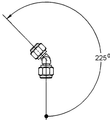
NOTE: Angular alignment shall be measured in degrees with a tolerance of  $\pm 2^\circ$ .
