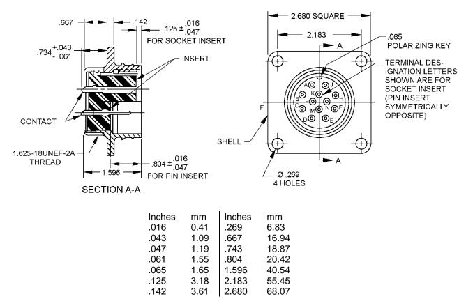
FIGURE 1. Connector, plug, electrical, intervehicular.
