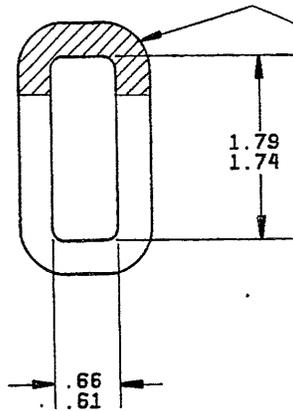
HARDNESS TEST TO BE PERFORMED IN SHADED AREA.
