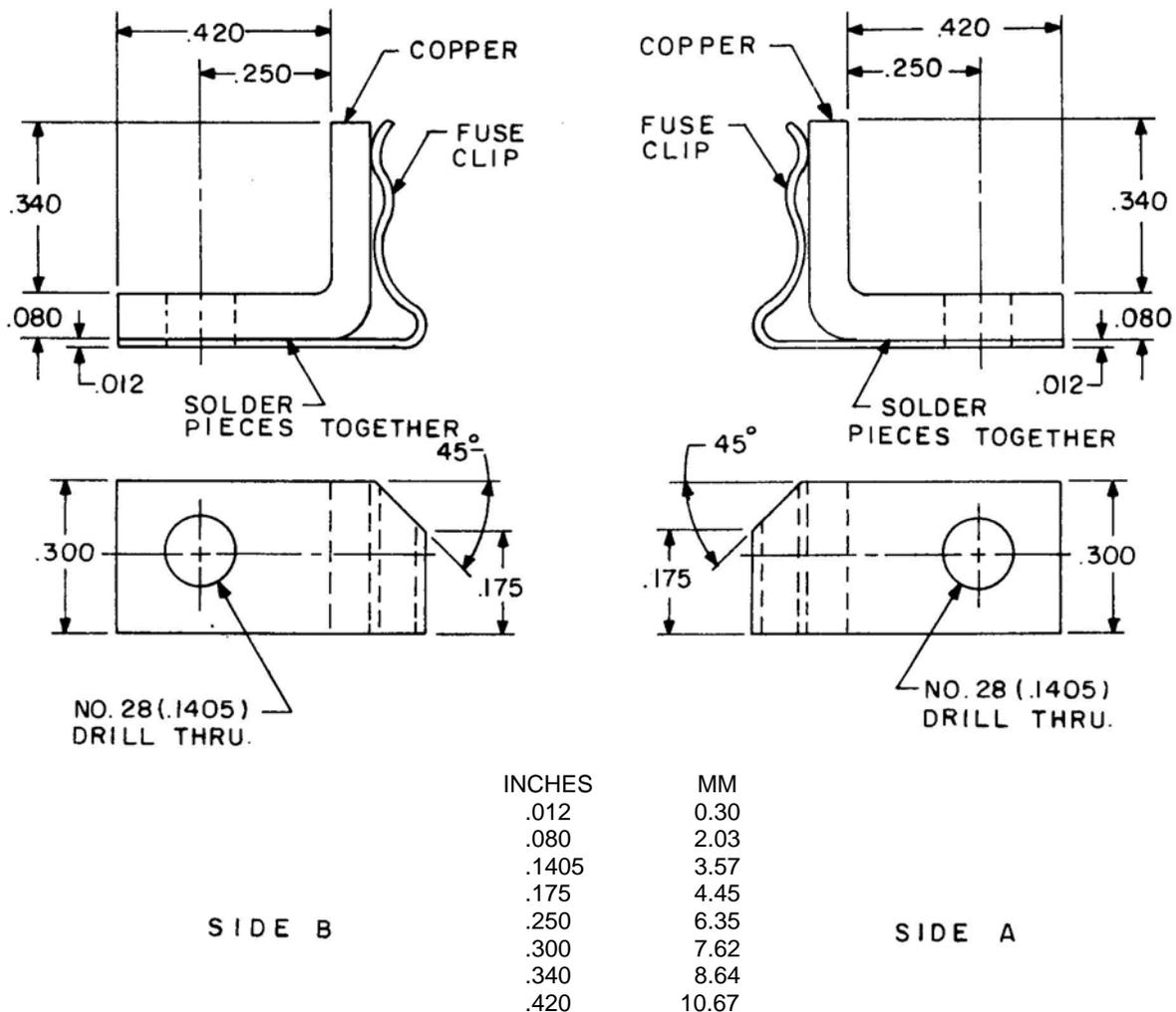
FIGURE 2. Test fixture for electrical measurements.
