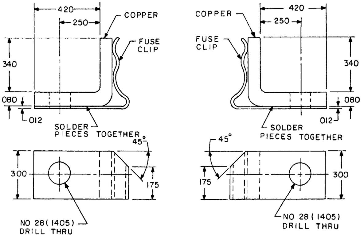
TEST FIXTURES FOR ELECTRICAL MEASUREMENTS
