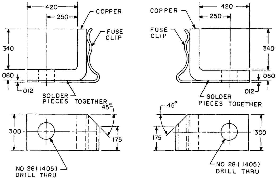
TEST FIXTURES FOR ELECTRICAL MEASUREMENTS
