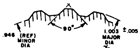
ENLARGED VIEW OF SERRATIONS
