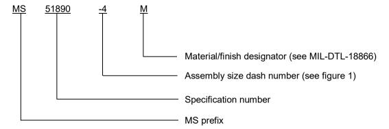
PIN example: MS51890-4M indicates a cap assembly, .3125 inch (7.938 mm), nickel-copper alloy.
