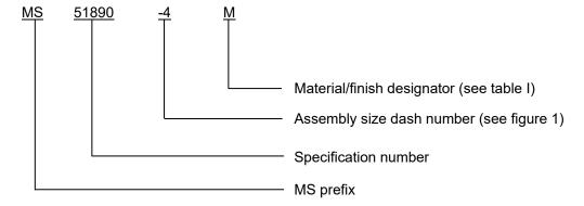
PIN example: MS51890-4M indicates a cap assembly, .3125 inch (7.938 mm), nickel-copper alloy.
