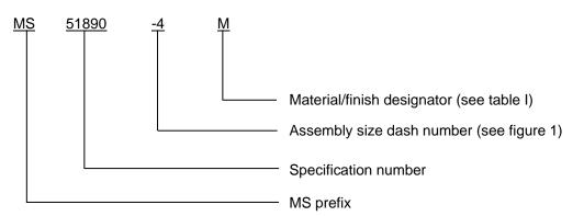
PIN example: MS51890-4M indicates a cap assembly, .3125 inch (7.938 mm), nickel-copper alloy.
