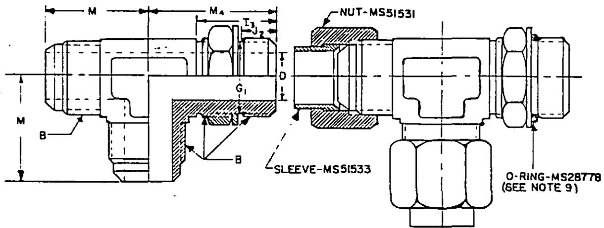
FIGURE 1. Elbow, Tube to Boss, Boss on Run, O-Ring, Flared.
