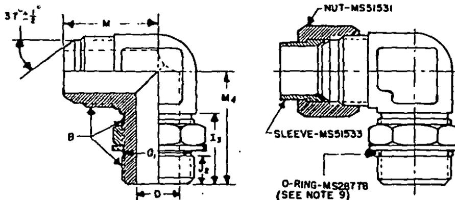
FIGURE 1. Elbow, Tube to Boss, 90 Degree, O-Ring, Flared.
