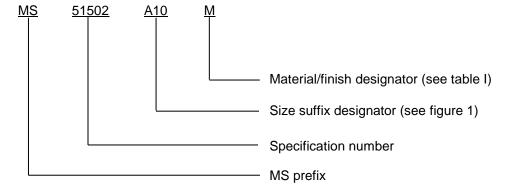
PIN example: MS51502A10M indicates a tube nipple, .6250 inch (15.875 mm), nickel-copper alloy.
