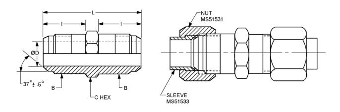
FIGURE 1. Nipple, tube, long.
